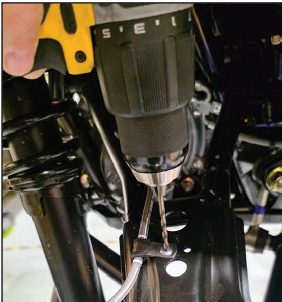
Drill out the rivets that connect the brake line to the rear control arms on both side.
