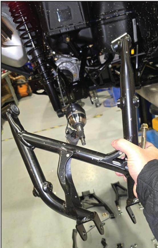
Remove the rear upper and lower control arms from both sides.
