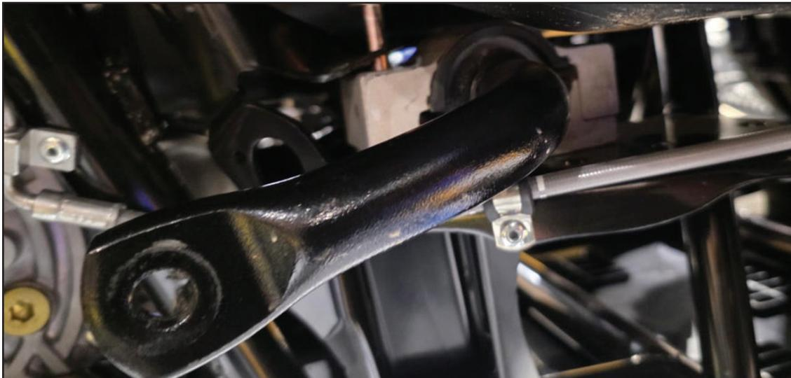
Disconnect the sway bar link from the control arm on both sides of the ATV.
