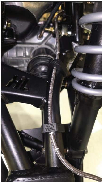
Secure the brake lines to the new arms using the brake line clamps. There are 6ea in a box, use three per side.
