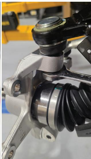
Disconnect the shock from the upper control arm and secure it out of the way.
