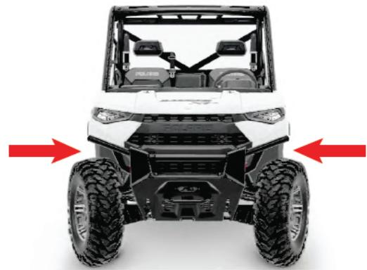
If the **FRONT OF THE WHEELS** are facing **IN**, adjust the tie rods **IN** or **REDUCE** the length of the tie rod.
