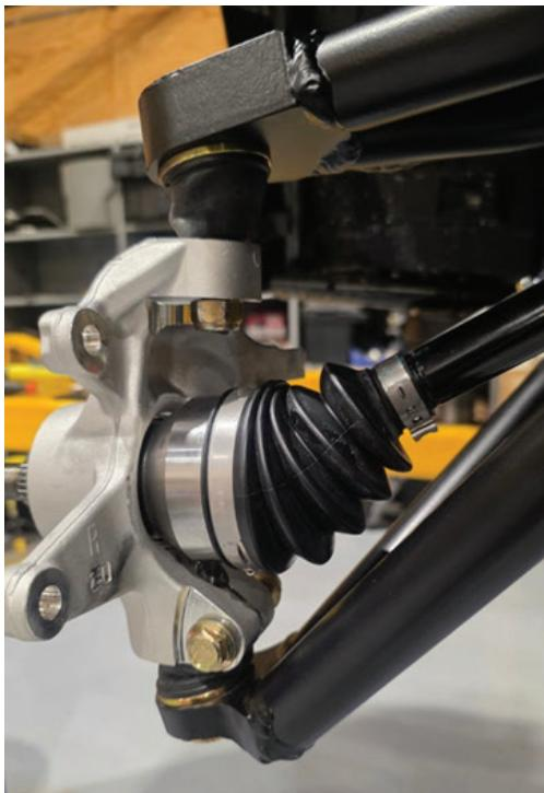
Connect the hub assembly to the new upper and lower control arms using the factory hardware.
