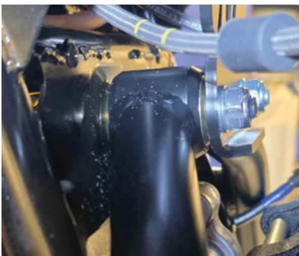
Next attach the upper control arms to the frame and fasten with the factory hardware.
