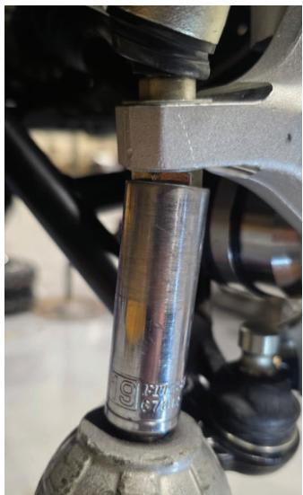
Remove ball joint nuts
