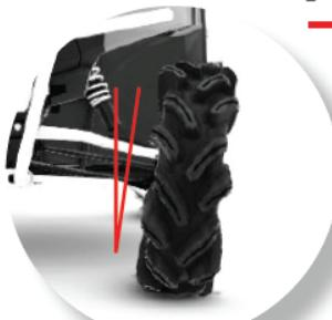
If you have a positive camber you will need to adjust the collar **OUTWARD** or lengthen the control arm. The maximum amount outward is "1.250" which could give up to 3° of negative camber.
