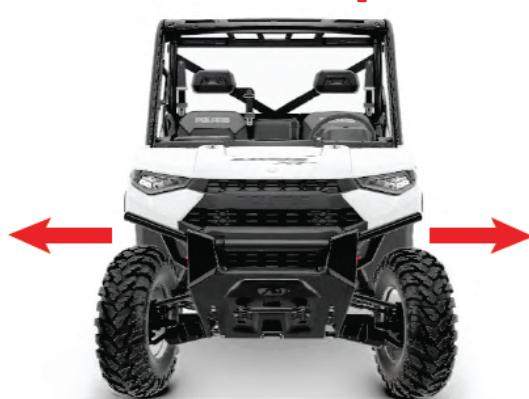
If the **FRONT OF THE WHEELS** are facing **OUT**, adjust the tie rods **OUT** or **INCREASE** the length of the tie rod.
