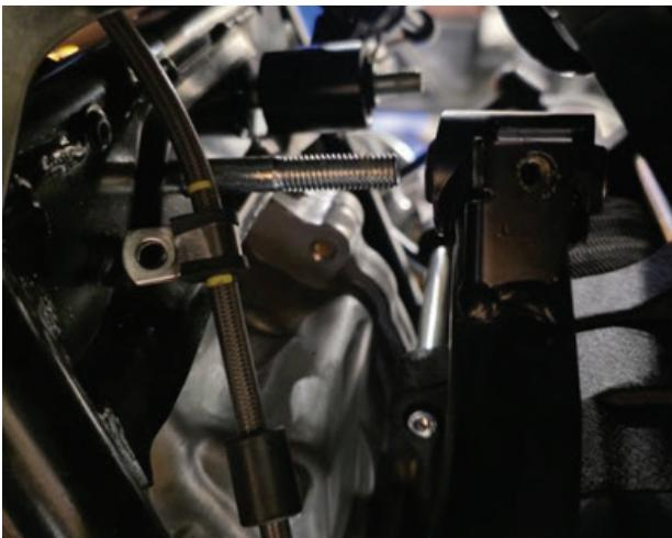
Disconnect the upper and lower control arms along with the sway bar links from the frame.
