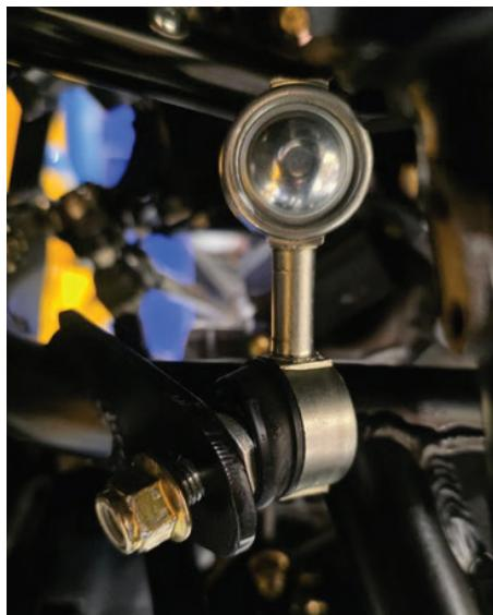
Connect the sway bar link to the control arms using the factory hardware.
