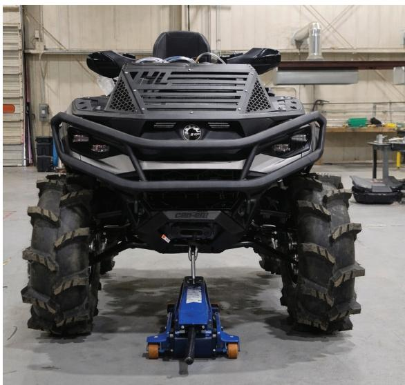
Place jack under center of ATV front end and lift until front wheels clear the ground. Be careful to support the ATV properly so that it is securely supported but so that Control arms and shocks can droop to full extension.
