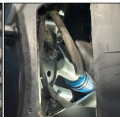
3: Install the Terrain Master Shock. Orientate the shock so the reservoirs are up and adjusters are facing out. *Note: If vehicle is heavy or using Long Travel, use outside mounting position*
