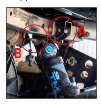
3: Reinstall the upper and lower shock hardware/bolt with Blue Loctite applied. Torque to factory specifications (Refer to your unit's owner's manual for the specification)
