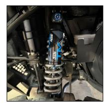
4: Reinstall the upper and lower shock hardware/bolt with Blue Loctite applied. Torque to factory specifications (Refer to your unit's owner's manual for the specification).
