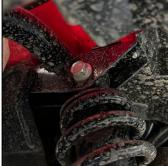
3: Install the Terrain Master Shock. Orientate the shock so the reservoirs are up and adjusters are facing out.
