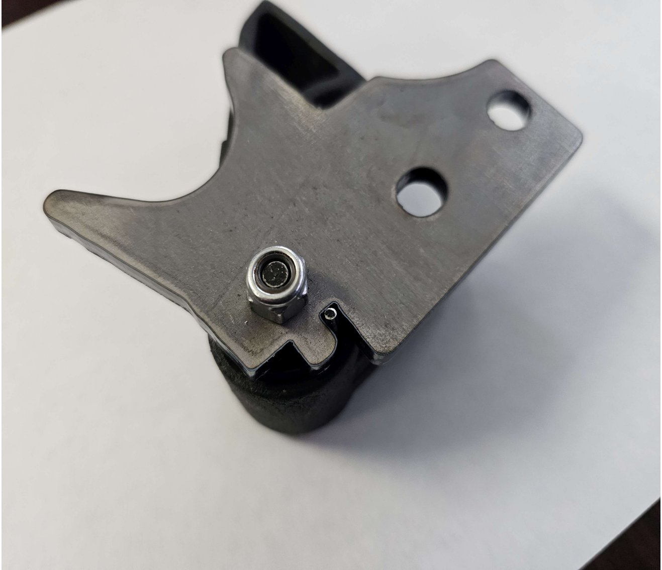
Seat latch spring recess and orientation
