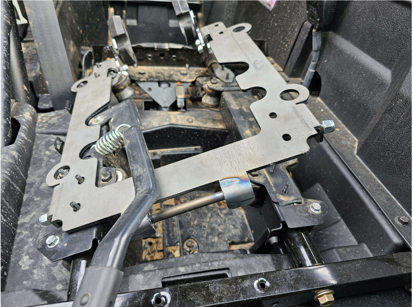
Seat base positioned onto rotated slider
