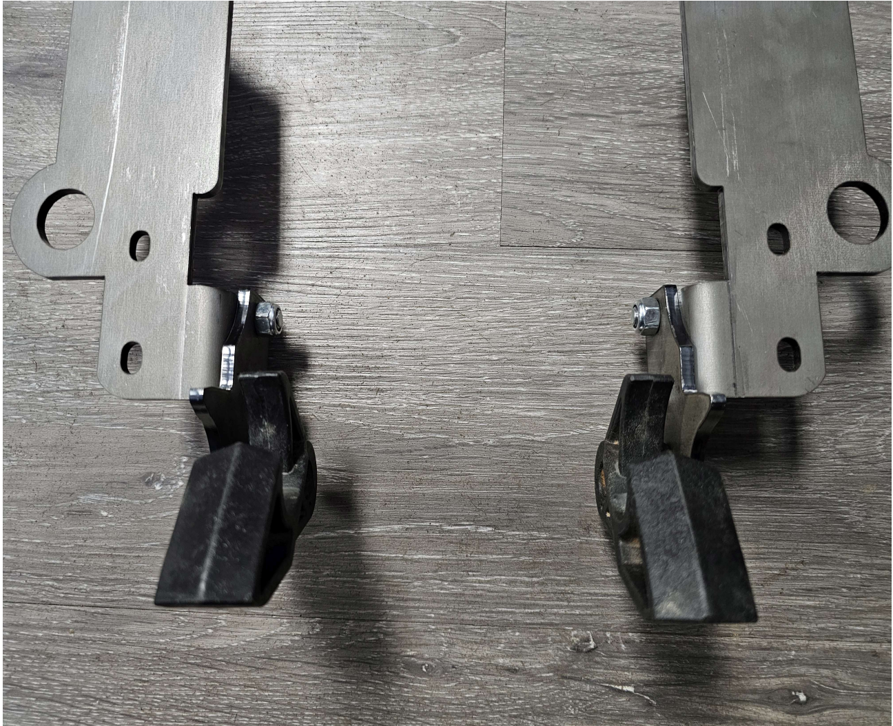
Seat latches installed onto Seat Base
