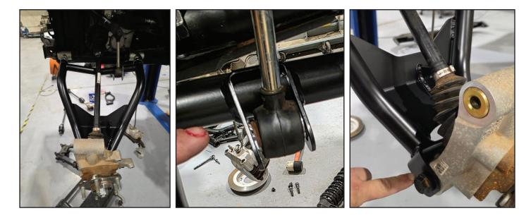
Attach the upper arm to the frame tabs and the hub assembly. Then attach the calipers back onto the hub assembly.
