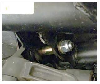
Note: Position the shock eyelet so that it is closest to the the front of the vehicle and the lock nut is always facing towards the rear.
