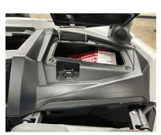
Open glove box lid. Using a T20 Torx remove four screws from glove box. Using a T40 Torx remove two screws from front dash.
