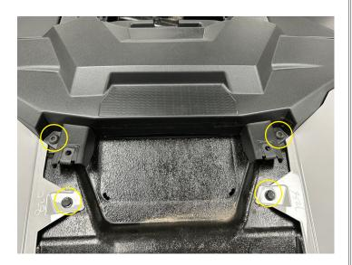
Carefully lift edge of left front fender to release from dash. Repeat process on right front fender.
