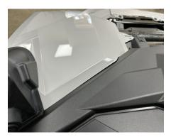
Carefully keep the front fenders elevated while tilting the dash panel up towards the seating area and slide toward the rear of the vehicle.
