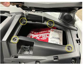
• Remove two T40 Torx screws from center of dash.
