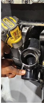
Locate the fuel tank vent line on the drivers side. Disconnect line from the frame under the ECU. Extend with the barb coupling and 36" of clear vent tubing. Later this line will be inserted into the vent line slot in the patented Warrior Riser.
