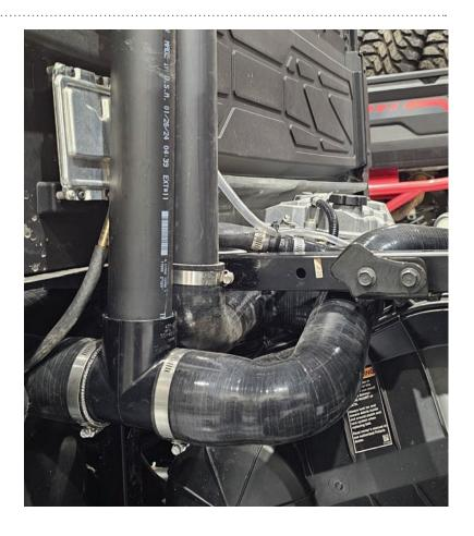
Insert SK-P-250 (16.5" long) into the belt box exhaust (right). Secure with #44 hose clamp.
