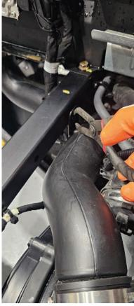
Connect the 3/4" ID hose to crankcase vent hose bar and secure with #12 hose clamp.
