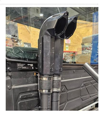
You will need to trim the bed around the new risers. Cut from the base of the bed vertically approximately 7.5" wide to clearance both riser pipes.
