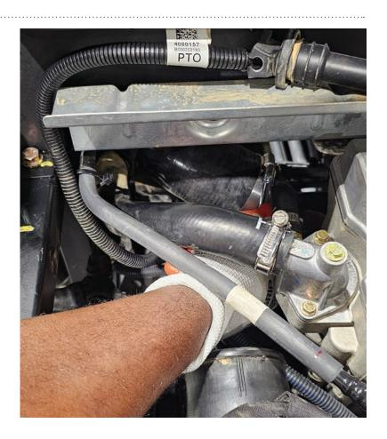
Connect the small end of the engine intake hose (71-12317) to the airbox with factory hose clamp. Connect the large end to the tee fitting and secure with another #44 hose clamp.
