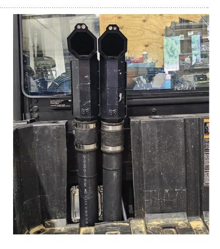
Place silicone boots (71-12300) on top of each riser pipe and secure with #44 hose clamp on each.
