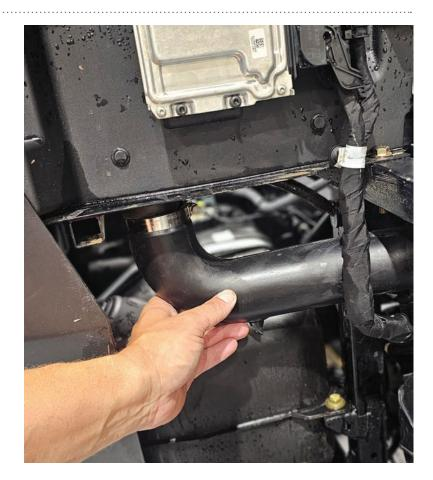
Remove clutch exhaust boot.
