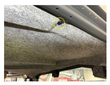
• Four Door Models: Remove a (2) T20 Torx screw on center rear headliner.
