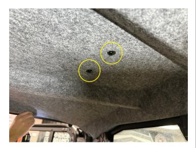
Remove T20 Torx screw on driver side rear panel.
