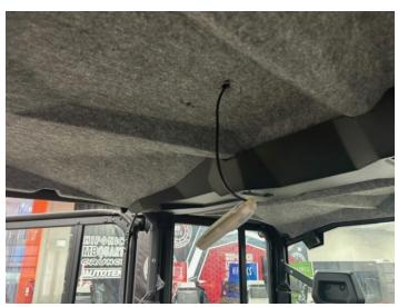
Four Door Models: Remove a T20 Torx screw on driver side headliner (if equiped). Repeat on passenger side.
