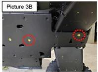
H. Align the center panels and tighten hardware. Install (24) 1/4-20 x 3/4" thread cutting screws (100108) and (24) supplied bowl washers (100087) shown in Picture 4.
