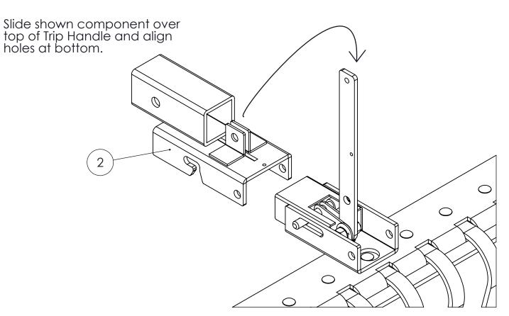
Secure Trip Handle and Bracket with Hardware shown below.
