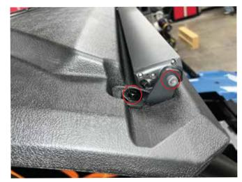
• Loosely install m8x30mm metal washer and M8 nylon locking nuts to front bolts.
