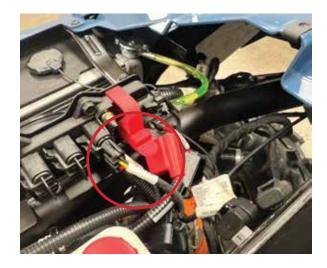
Crimp the fuse holder onto the main power wire. Connect the ring terminal of the fuse holder to the power lug on the Pulse network. Connect the ground wire to the negative lug on the Pulse network (like in the photo).
