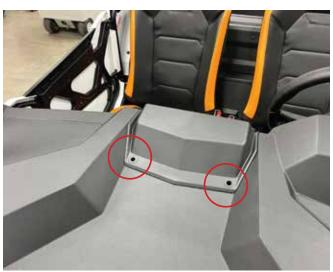
• Remove four bolts from the upper dash panel and remove panel.
