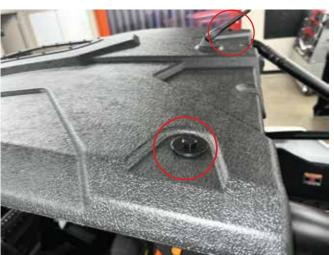
Install two center ROPS mounting brackets with m8x30mm bolts, M8x20 metal washers, M8x18 rubber washer, and M8 nylon locking nut.
