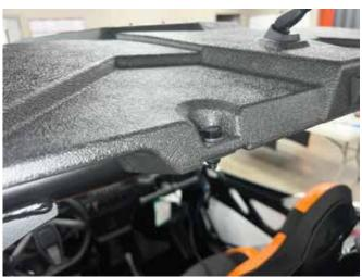
On the passenger side front corner of the ROPS there is a hole where you run your audio roof harness down.
