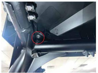
• Life the front of the OEM roof up and push towards the back of the vehicle to unclip the rear tabs. Then lift off.
