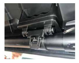
• Remove two bolts, one from each rear corner of the OEM roof.
