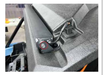
• Reinstall (2) M8x35mm bolts with M8x30mm metal washers and M8x26 rubber washers down through the lightbar. Install the rubber washer underneath the metal washer. Make sure they go through the ROPS.
