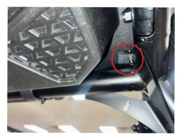
Loosely install two outer M8x40mm bolts, M8x35mm metal washers and M8x30 rubber washers down through the rear corner holes. Make sure they align with the speed clips.
