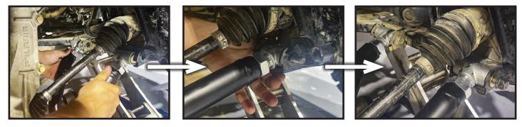
NOTE: BREAKING THE JAM NUT LOOSE WILL MAKE THE ARMS EASIER TO INSTALL. BE SURE TO RETIGHTEN THE NUT LATER.
