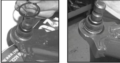
Use the factory nuts and bolts to connect the new A-arms to the frame. You will have left and right lower A-arms.
