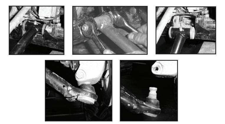
Remove the bushings, sleeves, and ball joints from the stock control arms. You will need to reuse these in the new forward a-arm kit.
