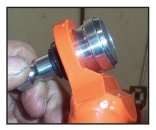
When pressing in the ball joint, support the ball joint end of the arm in a press with something solid below the arm and will allow the end of the ball joint to pass through completely. Be sure the support arm properly to allow the ball joint to pass through the hole straight and without interference. Again, be sure the boot will clear the fixture you are pressing into and the hole is deep enough for the full length of the ball joint to press into the arm.
