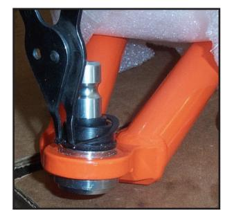
NOTE: IF THE BALL JOINT IS PRESSED IN TOO HARD IT WILL CRACK THE PAINT. IF THIS HAPPENS THEN TOUCH UP PAINT CAN BE APPLIED.
