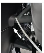
**Step 3:** With the wiring installed and the switch mounted, connect the harness to the OEM battery posts and check the functionality. With the light tested, and functional, secure any loose wiring, reinstall all the OEM trim pieces, and make any final adjustments to the angle of the light followed by tightening the hardware.
