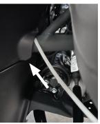
**Step 5:** With the wiring installed and the switch mounted, connect the harness to the OEM battery posts and check the functionality. With the light tested, and functional, secure any loose wiring and reinstall all the OEM trim pieces.
