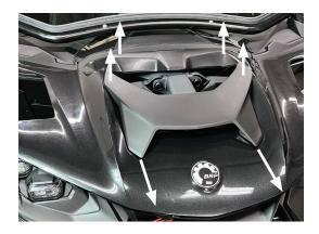
**Step 2:** Apply the sticky back EPMD and assemble the brackets.
