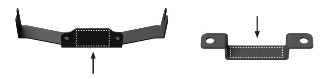
Next, loosely assemble one side of the bracket. Feed one of the 5/16 bolts through the washer, top bracket, spacer, bottom bracket, washer, and loosely secure it together with the 5/16 nut. Next install it on the shock tower with the arm of the bracket facing forward. Once complete install the hardware on the remaining side.
