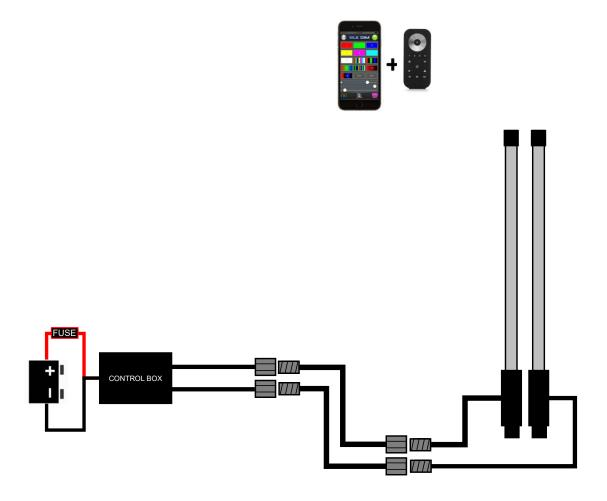
\*\*Controller needs to be mounted with in 10ft of whips (2 x 5ft extensions).
