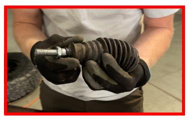
Reconnect the Axle Rod with boot to Billet Tie Rod Assembly.
