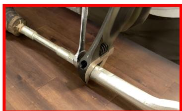
Take the new ZBROZ Tie Rod Assembly and remove the Axle Rod connection point completely.
