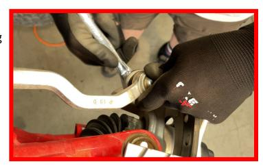
Remove the Zip-Tie holding the Tie Rod Boot in place located on the frame side.
