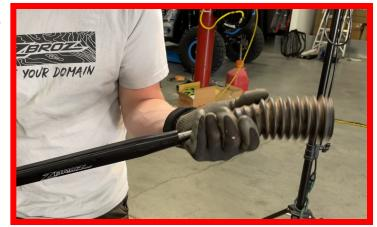
With a rag, clean the Axle Rod threads and apply medium Loctite.
