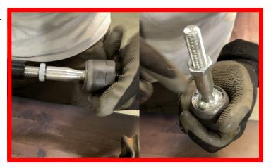
Slide the factory boot over the new ZBROZ Axle Rod exposing the Jam Nut.
