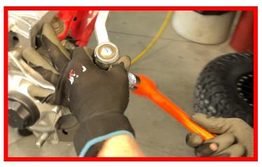
Remove the Axle Joint from the frame side connection using a large Crescent Wrench.
