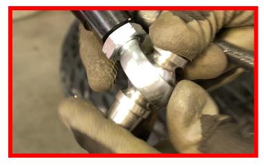
Insert the supplied 12mm bolt and Nut down through with the nut on bottom. Torque supplied bolt to factory specs.
