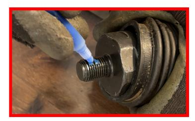
Thread the Axle Rod side into the PRO XP Frame. A trick to get it started is leaving the rod disconnected from the Axle Rod side. This will help make sure it is not cross threaded. Finish tightening with a large Crescent Wrench to factory torque specs.
