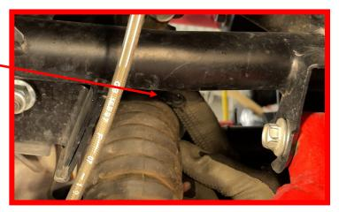
Remove the Tie Rod Bolt from the Spindle. NOTE: you may need to use a Hammer or Mallet to tap up on the bolt to dislodge it free.
