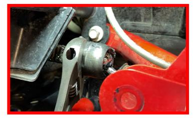
Using a Large Crescent Wrench and 16mm End Wrench, loosen the middle Jam Nut then continue to disconnect by turning it free by hand.
