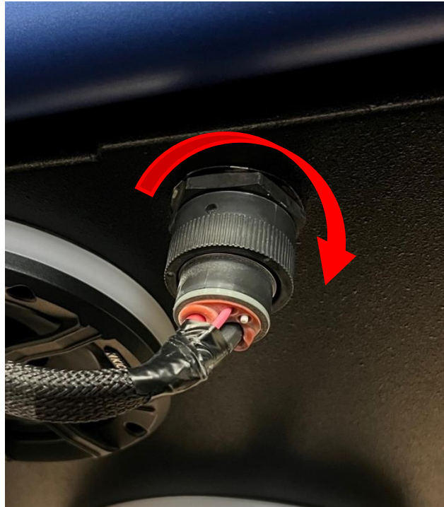
Figure 22: Align connector terminals and rotate 1/4 turn.
