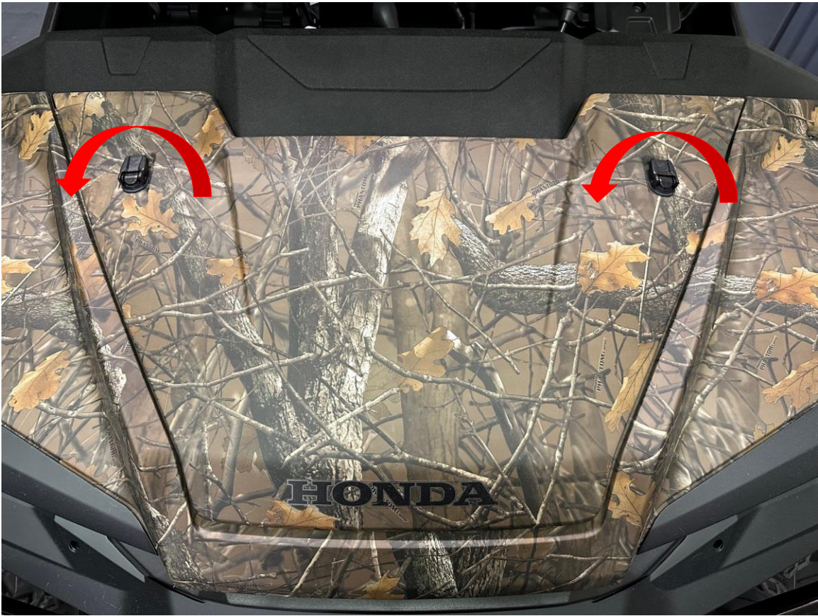
Figure 8: Remove the radiator hood access panel.
