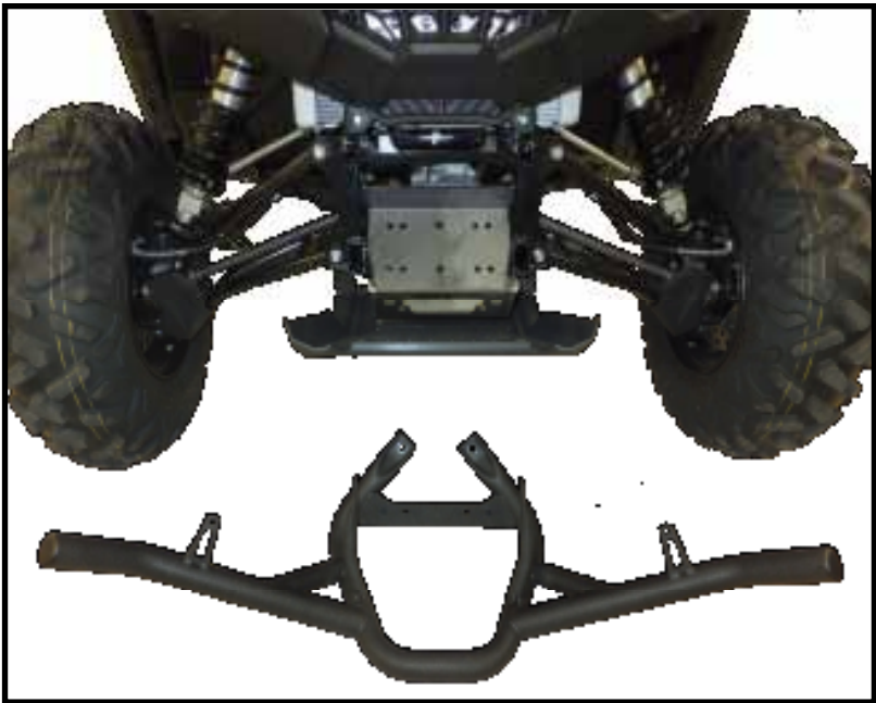
“Figure 6” Bumper Removed
