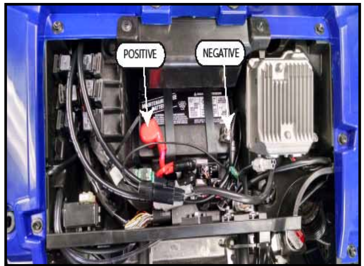
“Figure 12” Battery Location
