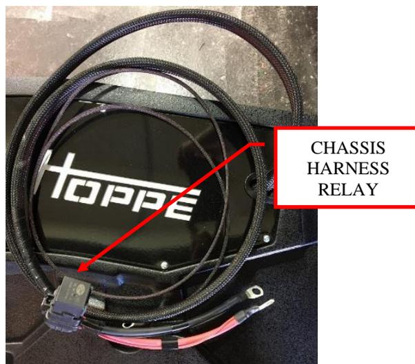
**Figure 1: Chassis harness relay.**
