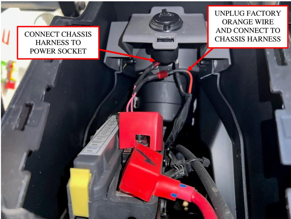
**Figure 13: Connect to the ignition wire.**
