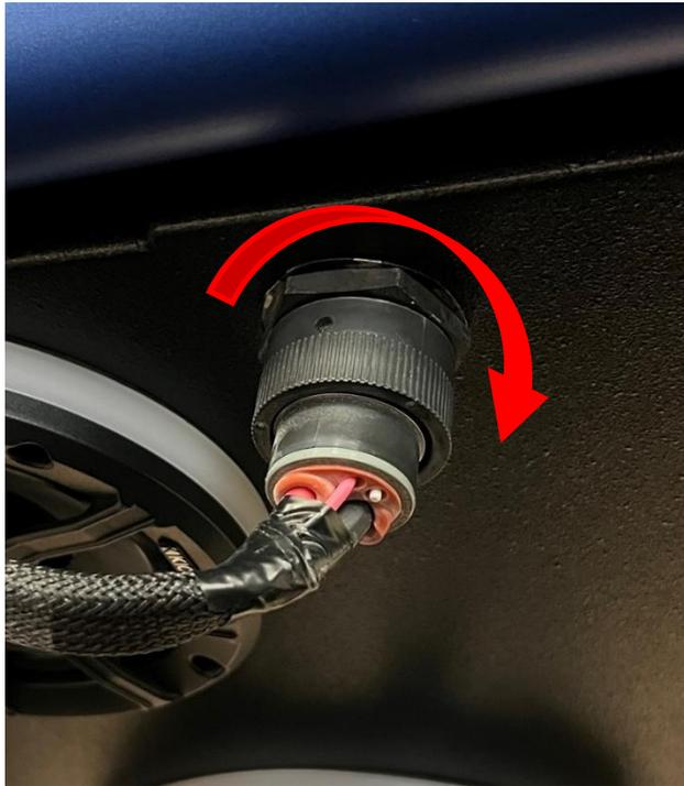
**Figure 14: Align connector terminals and rotate 1/4 turn.**
