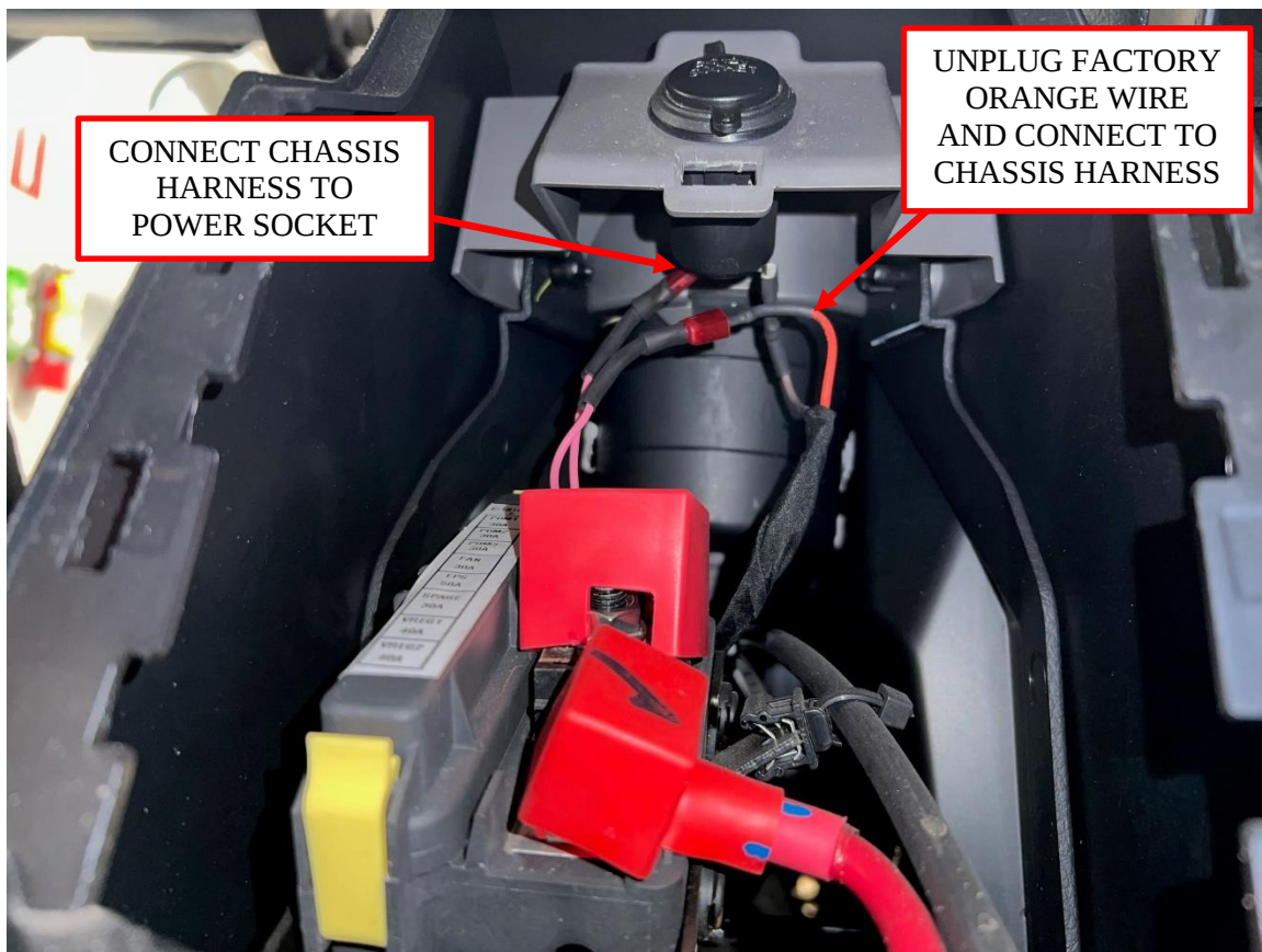
Figure 13: Connect to the ignition wire.
