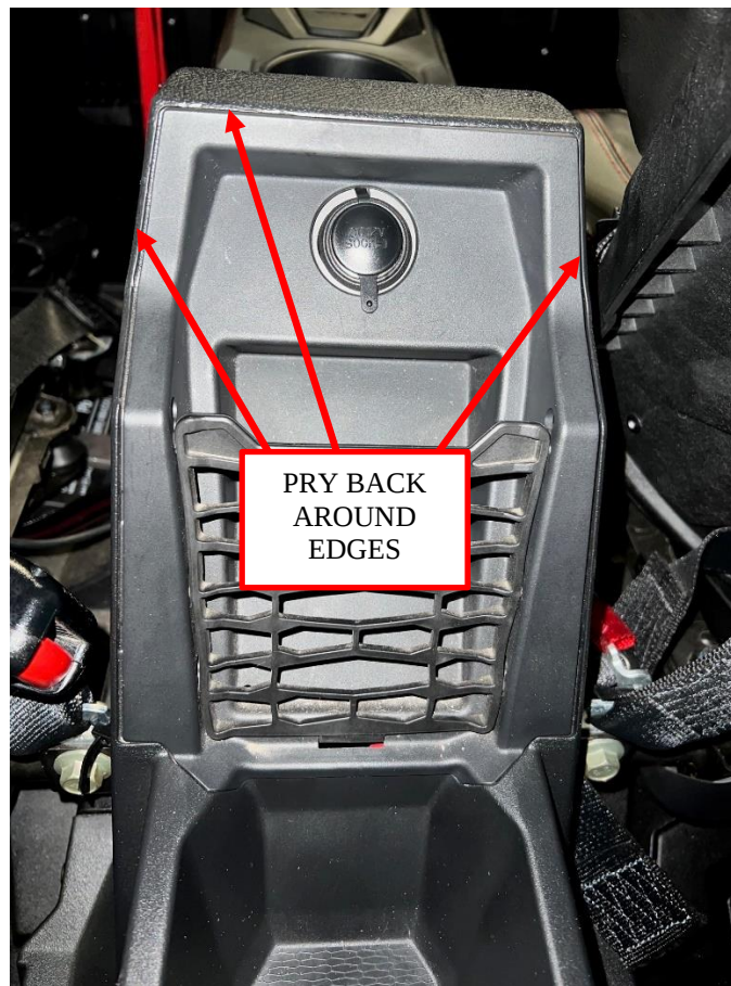
Figure 12: Remove trim panel from console.
