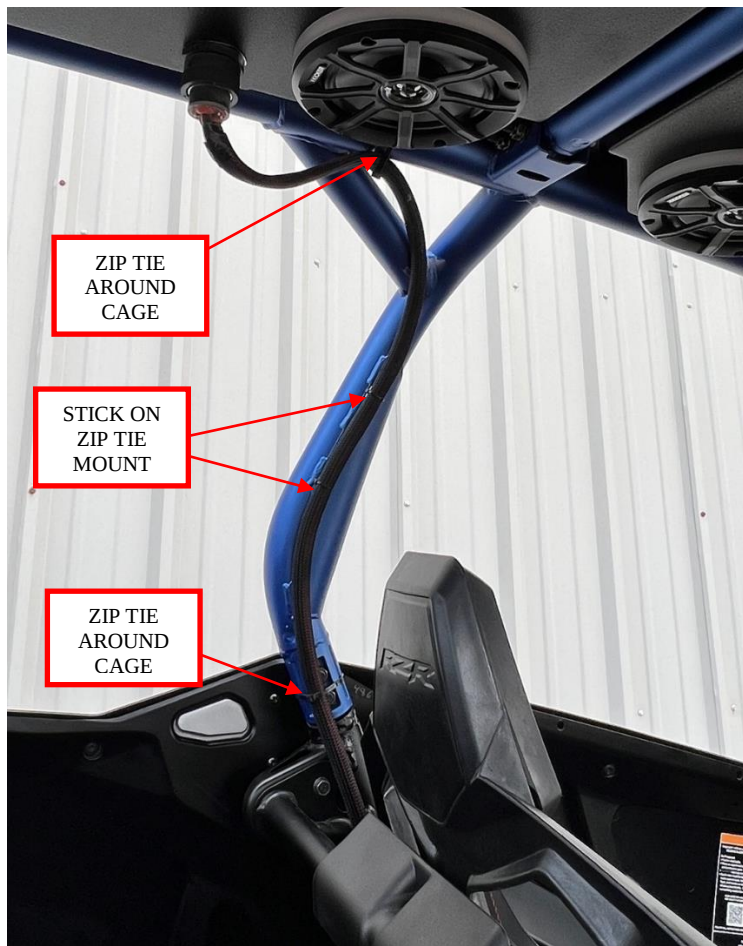
Figure 9: Route the chassis harness.
