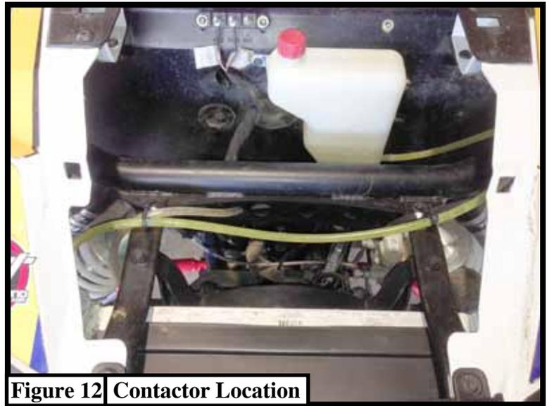
**Figure 12** Contactor Location
