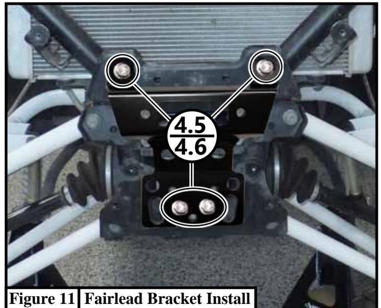
**Figure 11 Fairlead Bracket Install**
