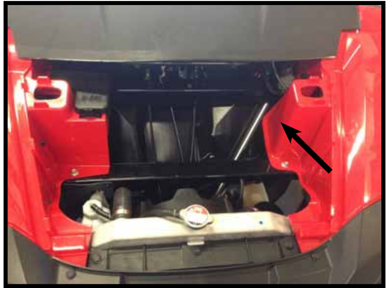
“Figure 7” Contactor Location
