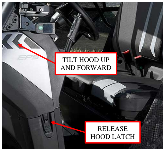
Figure 9: Tilt the hood to the front of the vehicle. Driver side shown. (Passenger side similar)
