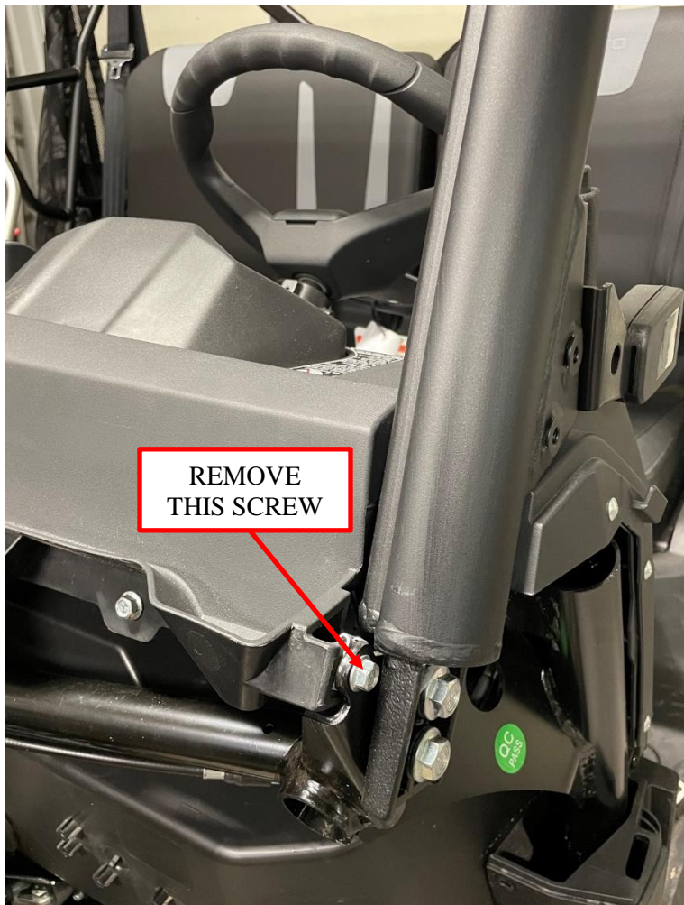
Figure 11: Remove the screw near the down tube. Driver side shown. (Passenger side similar)
