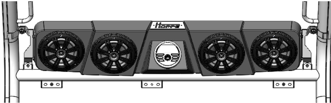
Figure 7: Loosely install the sound system on the mounting brackets.
