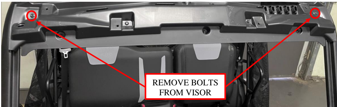
Figure 3: Remove the factory front visor bolts.
