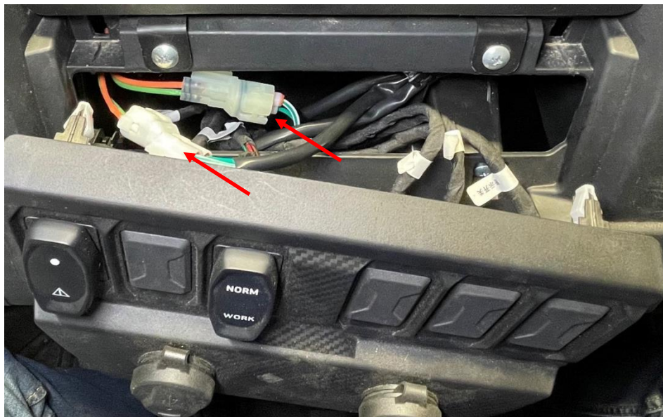
Figure 17: Connect the mating connectors from the chassis harness to the 12V power point connectors.
