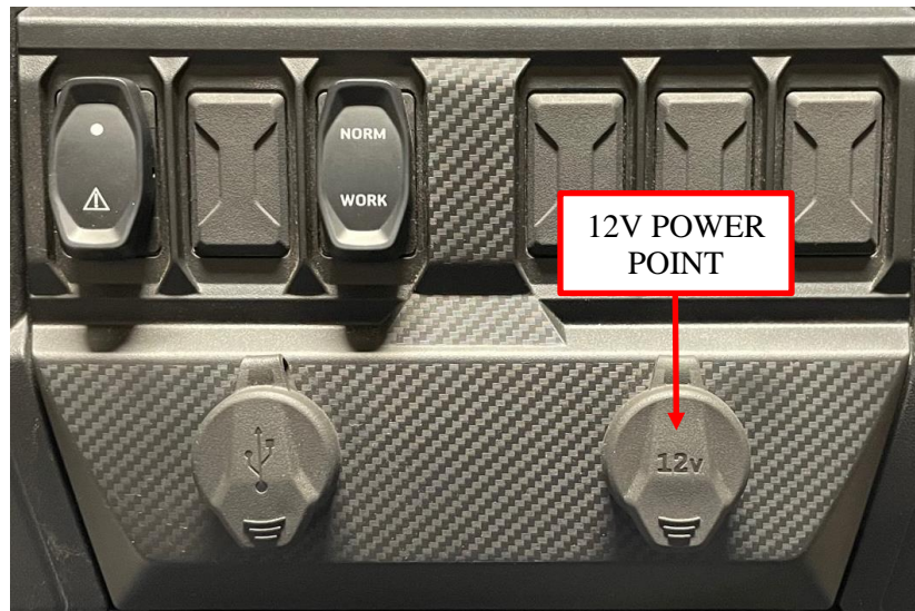
Figure 16: Connect the chassis harness to 12V power point connectors.
