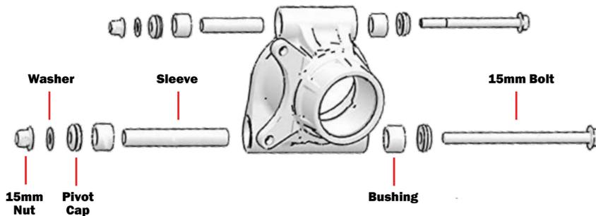
**NOTE:** Use caution when removing the bushings from the knuckle, there is a stop built in that prevents the bushing from pushing out when installed. Because of this, the bushing must be pushed out from the opposite side.
