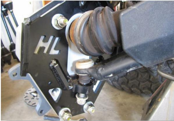
Loosely fasten all (4) bolts with 1/2" flat washers and 1/2" lock nuts. Ensure parts fit correctly then torque. (3/4) [105 ft lbs]
