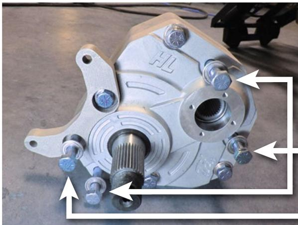
Insert the washers and bolts below through the remaining (4) holes in the rear portal box.
