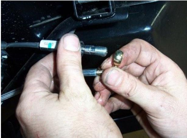
Install the 58" FRONT RIGHT brake line to the banjo bolt. Run the line back through the frame and to the RIGHT (PA) side hub.
