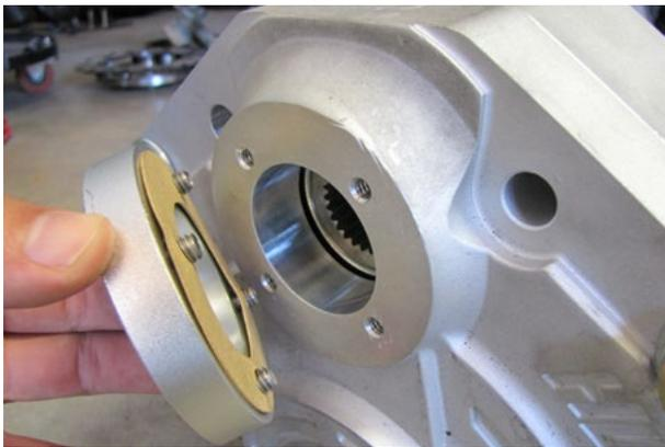
Remove the 1/4-20 x 3/4" screws, cap, and gasket from the lid of the assembled portal box.
