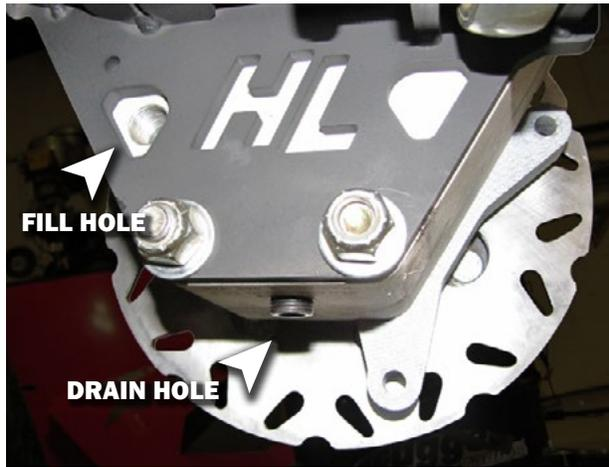
1. Ensure the vehicle is positioned securely and 'Level'.
