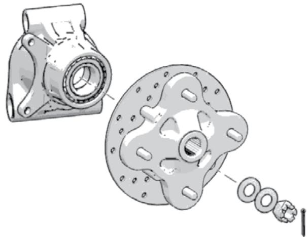
Remove the cotter pin and castle nut (27mm) on the rear axles, then remove the brake rotor assembly.
