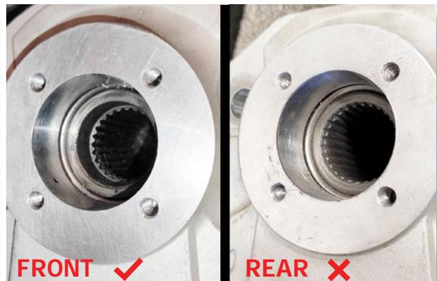
**NOTE:** On the FRONT portal boxes, the drive gear splines should be recessed to accommodate the shorter front drive shaft splines.
