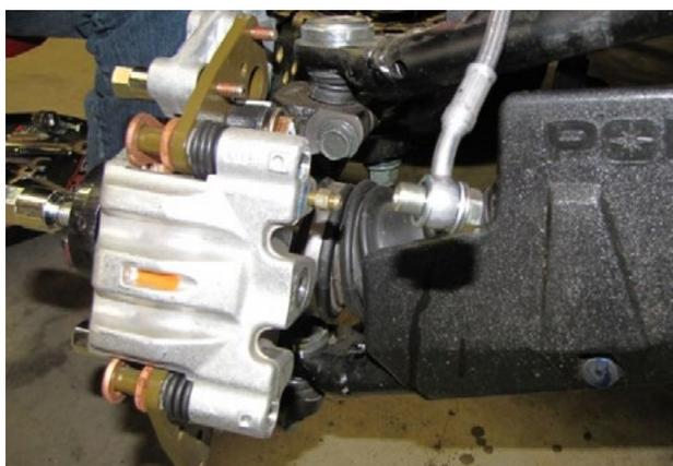
Disconnect the stock brake line from the caliper, if you have not done so already.
