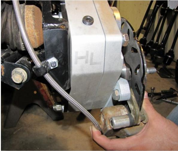
Reattach the brake line to the caliper.
