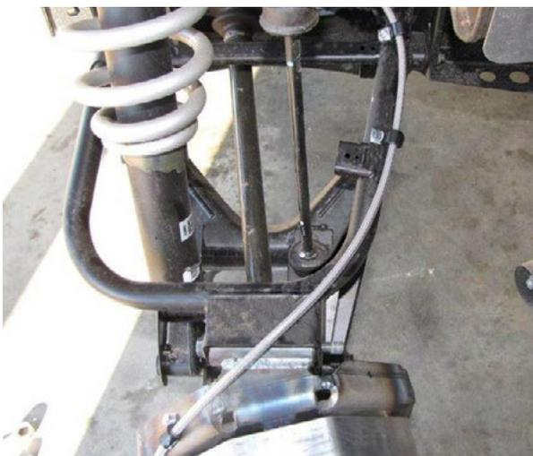
**NOTE:** ENSURE THAT THERE IS NO BINDING, PINCHING, OR INTERFERENCE WITH MOVING PARTS AND THE NEW BRAKE LINES.
