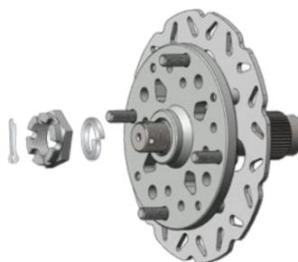
Slide on the 30mm lock washer, 30mm castle nut. (46mm) [Min 120 ft lbs]
