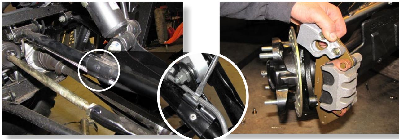
Disconnect brake lines from arms and frame. Remove the brake caliper mounting bolts (15mm) Remove the front mud scraper (8mm). **KEEP ALL FACTORY HARDWARE.**
