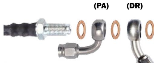
The factory brake line banjo bolt should be in this sequence: bolt, washer (PA) brake line, washer (DR) brake line, and washer.
