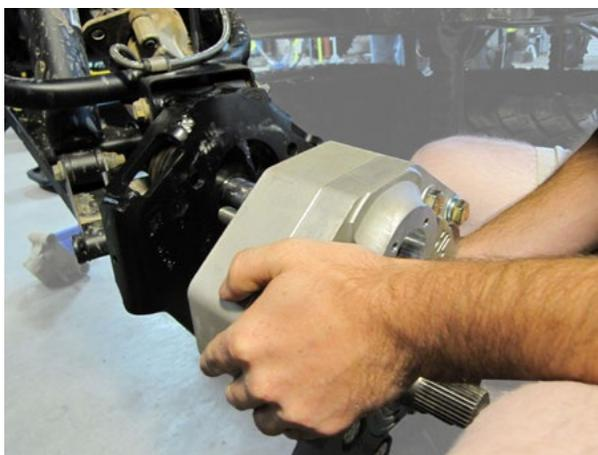
Apply water-resistant grease to the drive splines. Be sure to apply product all around the outer edge as well.
