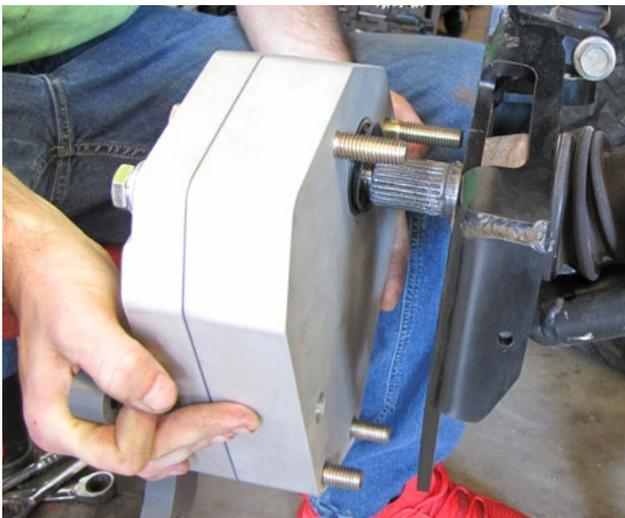
Apply water-resistant grease to the drive splines. Be sure to apply product all around the outer edge as well.
