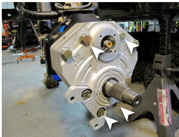
Loosely fasten all (4) bolts with 1/2" flat washers and 1/2" lock nuts. Ensure parts fit correctly then torque. (3/4) [105 ft lbs]
