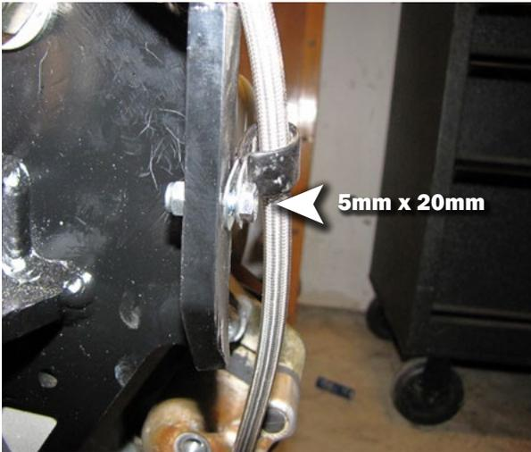
Secure the line to the portal backing plate using a p-clamp and the 5mm x 20mm bolt, 5mm washer, and 5mm lock nut.
