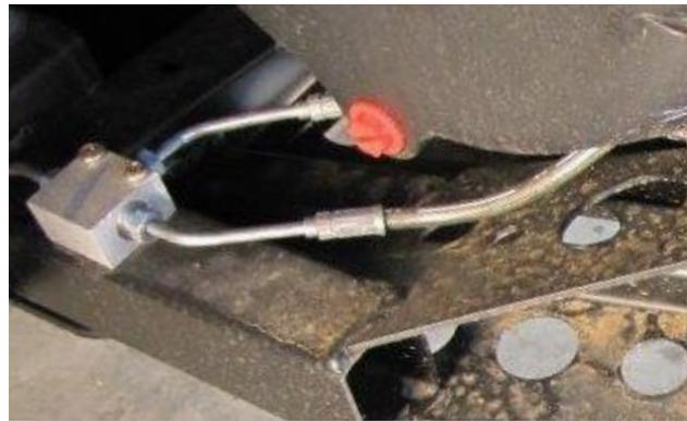
Install the new 63" REAR RIGHT brake line to the block, then the 55" REAR LEFT line.
