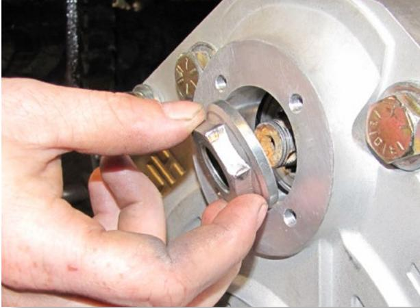
With the portal box installed, apply **LOCTITE (BLUE)** to the supplied **M18 axle nut PGLC-AXNUT-2** and torque onto the drive shaft axle. (30mm) [20 ft lbs]
