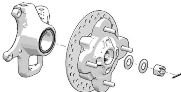
Remove the cotter pin, axle nut, and washers from the hub assembly, then remove the hub. (27mm)
