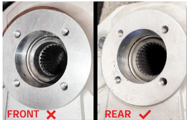
**NOTE:** On the REAR portal boxes, the drive gear is reversed, and the splines should be to the outside edge to accommodate the longer rear drive shaft splines.
