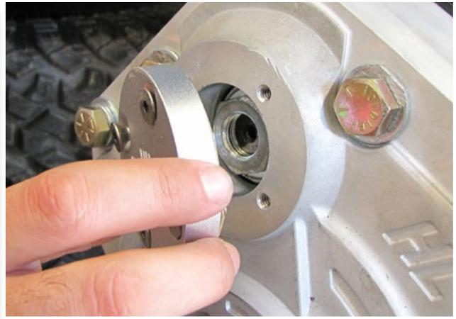
Align the portal box lid cap & gasket. Use the **1/4-20 x 3/4"** screws and install the cap to the portal box. [8 ft lbs]
