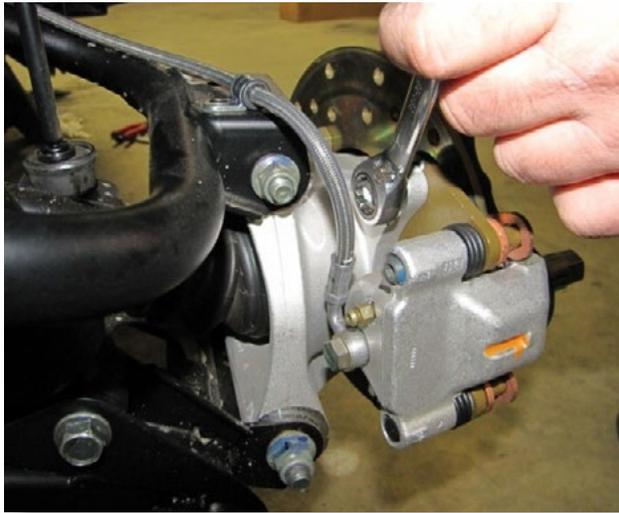
Remove the brake caliper mounting bolts from the hub assembly. (15mm) **KEEP FACTORY HARDWARE.**
