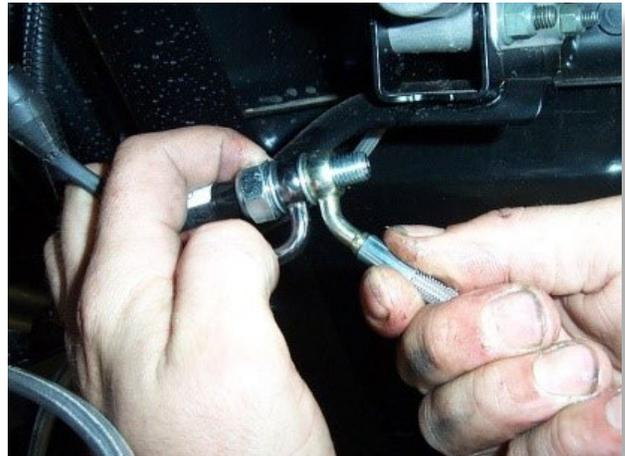
Install the new 50" FRONT LEFT brake line to the banjo bolt. Run the line back through the frame and to the LEFT (DR) side hub.
