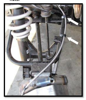
j. If you are <u>using aftermarket upper arms</u>, secure any remaining brake lines with **zip ties**. Make sure there is no binding in the lines once they are secured.
