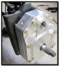
d. Loosely fasten the all six bolts with 1/2" flat washers and 1/2" lock nuts. Recheck all parts that were used and make sure everything fits correctly, and then go ahead and fasten all bolts. (3/4)[105 ft lbs]
