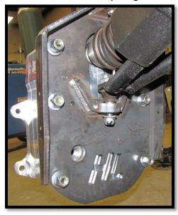
e. Install the tie rod end into the backing plate tie rod mount bracket. Fasten the tie rod end with the factory hardware. (18mm)[90 ft lbs]
