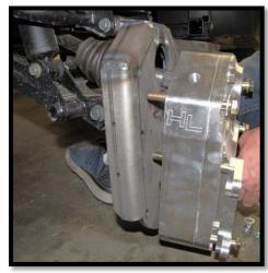
d. Loosely fasten the all four bolts with 1/2" flat washers and 1/2" lock nuts. Recheck all parts that were used and make sure everything fits correctly, and then go ahead and tighten and torque all bolts. (3/4)[105 ft lbs]
