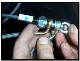
c. Install the new **58" FRONT RIGHT** brake line to the banjo bolt. Run the line back through the frame and to the (PA) side hub.
