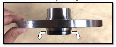
c. With the shorter lip side faced down, find the bolt pattern that corresponds to your make and model. Use the provided studs PGLC-WSTUD-102 (12mm-1.5 stud) (4/156mm bolt pattern)
