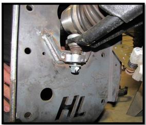
Insert the drive shaft into the backing plate. Then place the upper ball joint into the upper ball joint mount bracket. Fasten it with the factory hardware. (15mm)[50 ft lbs]
