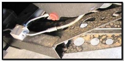
f. Route the brake lines back to their corresponding hubs. They will need to be routed down the same passage where the factory lines were.
