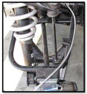
g. Reattach the brake line to the calipers.
