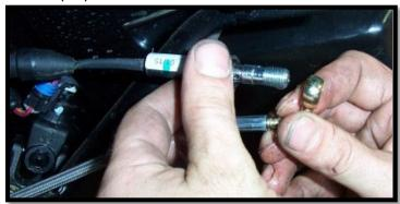
d. Install the new **50" FRONT LEFT** brake line to the banjo bolt. Run the line back through the frame and to the (DR) side hub.
