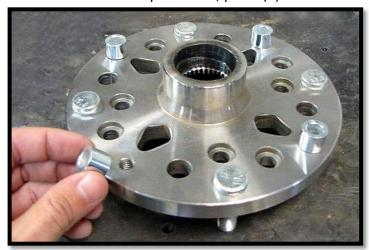
f. Locate a **brake rotor PGLC-ROTOR-3**. Place the rotor on to the hub and line the holes up with the rotor spacers and tapped holes.
