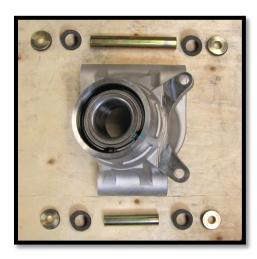
c. Insert the bushings, pivot tubes, and pivot caps into the collars of the **rear right backing plate (91R-R). NOTE**: We recommend applying good water-resistant grease to the bushings and especially the pivot tube. This will help prevent excessive friction & wear plus add longevity to the life of the bushings and pivot tube.
