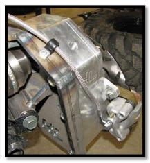
If you are <u>using factory upper arms</u>, you can re-use the factory p-clamp locations to install new supplied p-clamps. Secure them to the upper arm using 5mm x 16mm bolts, followed by 5mm washers and 5mm lock nuts.
