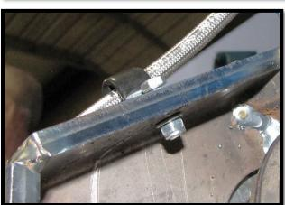
h. Use the factory A-arm clips and the supplied **zip ties** to reposition the brake lines, then fasten the brake line back to the caliper. **Make sure there's no binding in the lines, even at full turn.**
