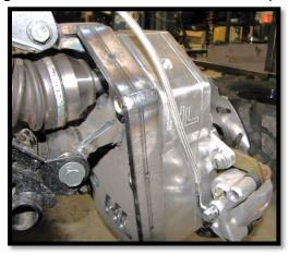
h. Slide a **p-clamp** over the brake line. Secure it to the rear backing plate using a **5mm x 20mm bolt** through the clamp and backing plate, followed by a **5mm washer** and **5mm lock nut.**
