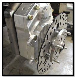
b. Slide on the supplied **30mm lock washer**, followed by the **30mm spindle castle nut**. (46mm) [Min 120 ft lbs] Tighten the castle nut further if needed to align grooves with holes in the spindle for the cotter pin. Install the supplied **cotter pin**. Both ends of the cotter pin must be folded.
