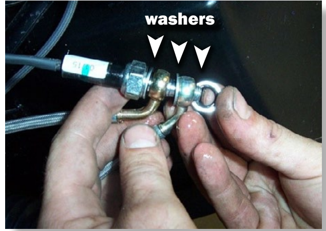
Save the factory washers that separate the two front lines. Remove the line from the UTV.
