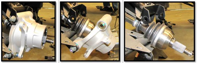
f. While you have the knuckle removed and have more access to the arms. You will need to drill/remove the rivets of each p-clamp. Doing this now will make the new rear brake line installation easier later.
