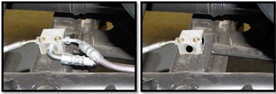
c. Install the new **74**" **rear right** (pass. side) brake line to the t-block. It will need to be routed down the same passage where the factory line was.
