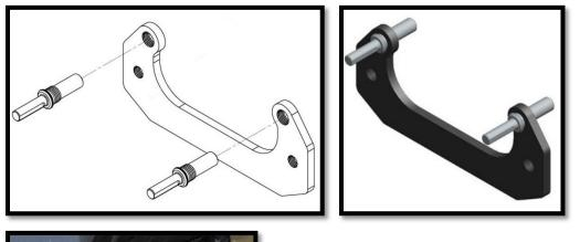
Install the caliper onto the portal box between the new caliper bracket and rotor. Use the factory mounting bolts. Position brake line banjo fitting so it runs at the proper angle for maximum suspension travel. Tighten & torque to specifications. (15mm) [30 ft lbs]
