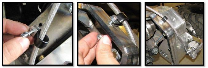
g. Secure the brake lines by using new p-clamps (WL-CLAMP-12). Secure them 5mm x 16mm bolts, 5mm washers, and 5mm lock nuts. Use zip ties to secure any remaining slack or aftermarket arms. Make sure there is no binding in the lines once they are secured.
