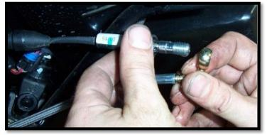
d. Install the existing factory (PA) side brake line and install it to the banjo bolt. This is replacing the factory (DR) side brake line.
