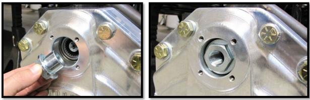
c. Align the portal box lid cap & gasket. Use the **1/4-20 x 3/4**" screws and install to the box. (3/16) [8 ft lbs]
