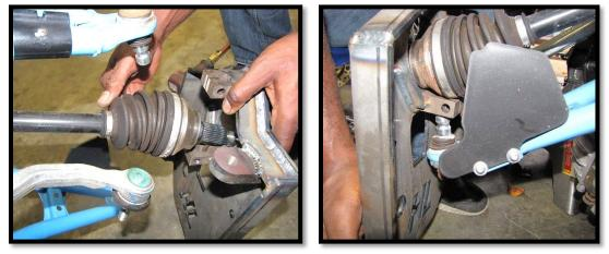
c. Insert the drive shaft into the backing plate. Then place the upper ball joint into the upper ball joint mount bracket. Fasten it with the factory hardware. (15mm) [50 ft lbs]
