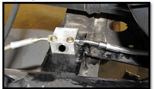
d. Before installing the new **60" rear left** (driver side). First install the 3/8 adapter. The arched end should face out once installed. Now attach the brake line to the adapter.
