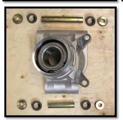
c. Insert the bushings, pivot tubes, and pivot caps into the collars of the rear right backing plate (117D-R).
