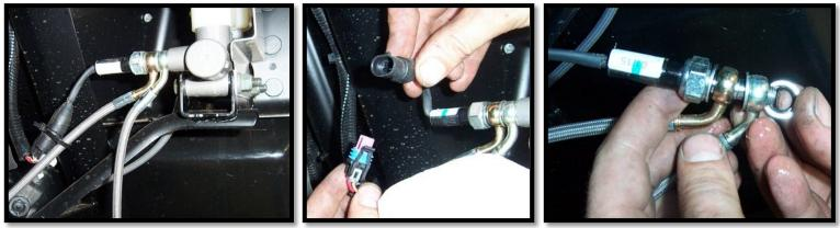
c. Install the new **(64Y) 56" FRONT RIGHT** brake line to the banjo bolt. Run the line back through the frame and to the (PA) side hub.
