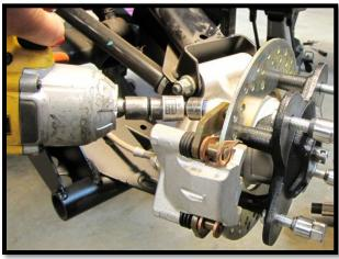
b. Remove the caliper from the rear hub. It is not necessary to remove the brake line from the caliper at this time. Leave the brake hose attached to the caliper and hang the calipers out of the way. Take precautions to ensure the brake hose isn't stretched or pinched.
