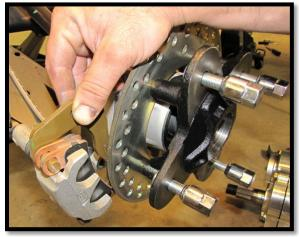
c. Remove the cotter pin and loosen the rear wheel hub castle nut (27mm). Remove the nut from the rear wheel hub assembly. Then remove the brake rotor assembly.
