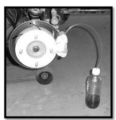
slowly open the caliper bleeder screw 1/4" turn so the air and fluid will displace into the container.
