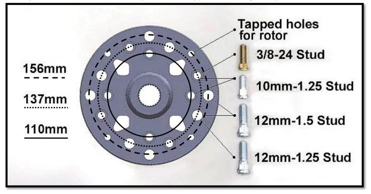
d. You can use a press to install the studs. You can also use large sockets as spacers to press them in. Take care not to press the studs into the threaded tapped holes for the rotor!
