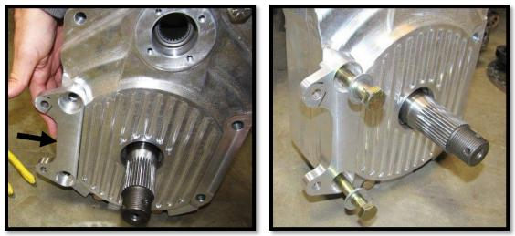
d. Slide a 1/2" flat washer onto (4) 1/2 x 4-1/2" bolts and insert them into the remaining four holes of the box.
