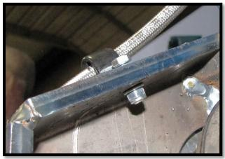
h. Use the factory A-arm clip and supplied p-clamps to secure the brake lines to the factory arm and frame. Then fasten the brake line back to the caliper. Use a 5mm x 16mm bolt, 5mm washer, and 5mm lock nut for the arm. Then use a #10x3/4 self-tap screw to secure the p-clamp to the frame. <u>Make sure there is no</u> <u>binding in the lines, even at full turn</u>. Use zip ties to secure any remaining slack or aftermarket arms.
