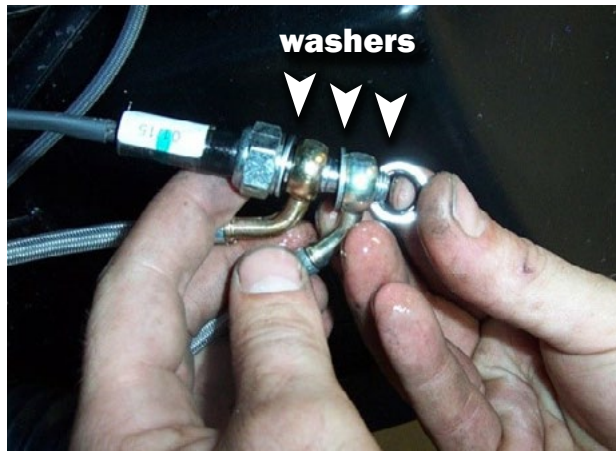
Save the factory washers that separate the two front lines. Remove the line from the UTV.
