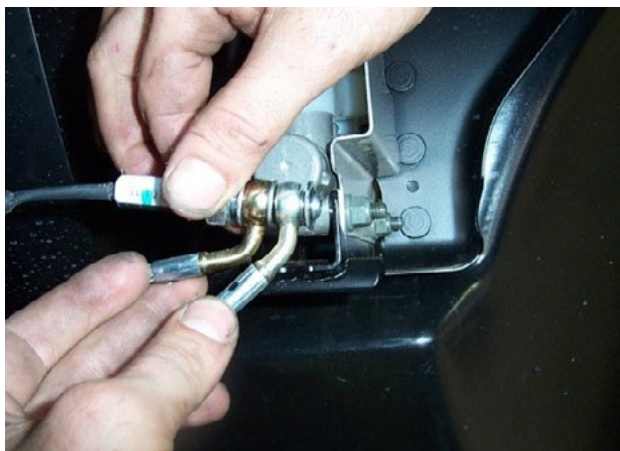
Disconnect the banjo bolt and brake lines from the master cylinder.
