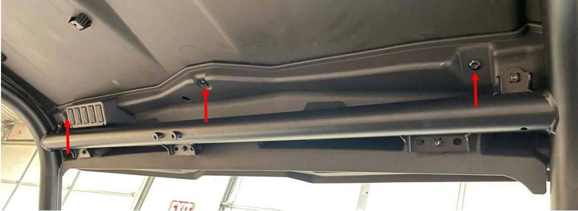
Figure 2: Remove the front bolts securing the roof to the visor.
