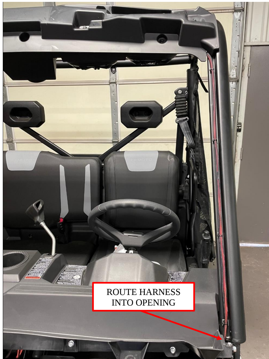
Figure 13: Chassis harness routing up the front down tube.
