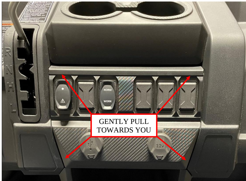
Figure 14: Remove the center section of the dash.
