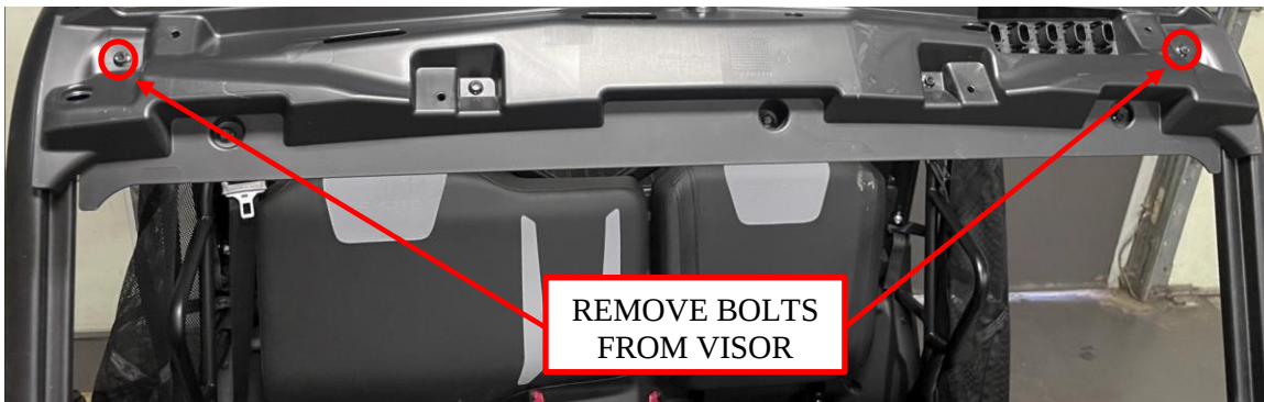
Figure 3: Remove the factory front visor bolts.
