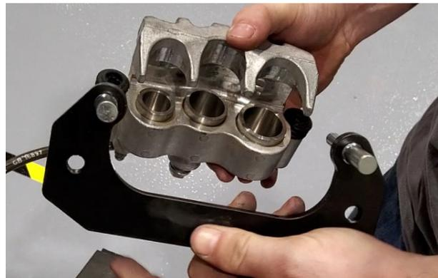
Install the supplied hanger bracket (108M) to the caliper. **REINSTALL BRAKE PADS.**
