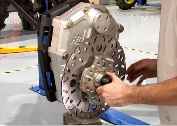
Slide on the **30mm lock washer**, **30mm castle nut**. (**46mm**) [Min **120 ft lbs**] Tighten the castle nut further if needed to align grooves with hole in the spindle for the cotter pin. Install the cotter pin, then bend it to secure it.
