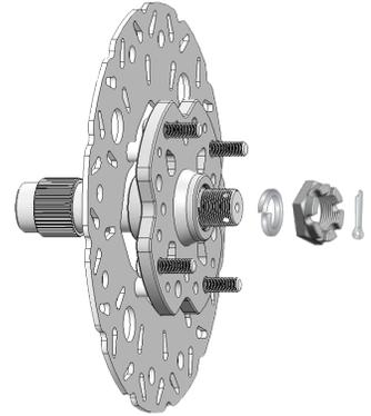
Apply waterproof grease to the spindle splines and slide the brake rotor assembly onto the spindle shaft.
