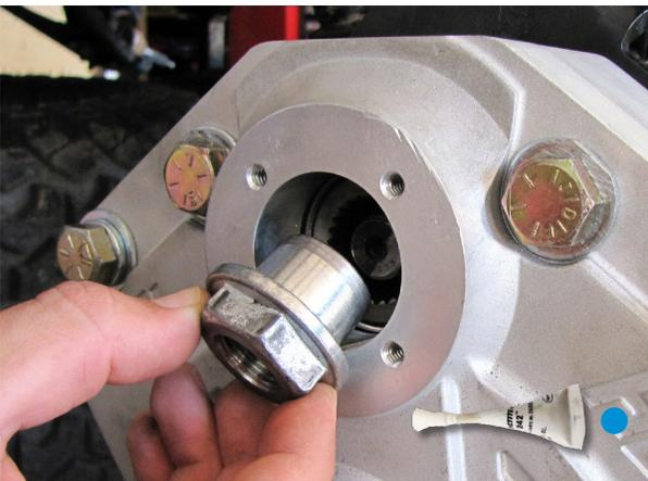
**With the portal box installed, apply LOCTITE (BLUE) to the supplied M18 axle nut PGLC-AXNUT-4 and torque onto the drive shaft axle. (30mm) [20 ft lbs].**
