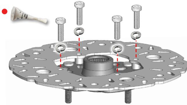
Install the rotor and secure it to the hub by applying **LOCTITE (RED)** to the (4) 3/8 x 1-1/4" hex head bolts & (4) 3/8 lock washer (7/32) [45 ft lbs].
