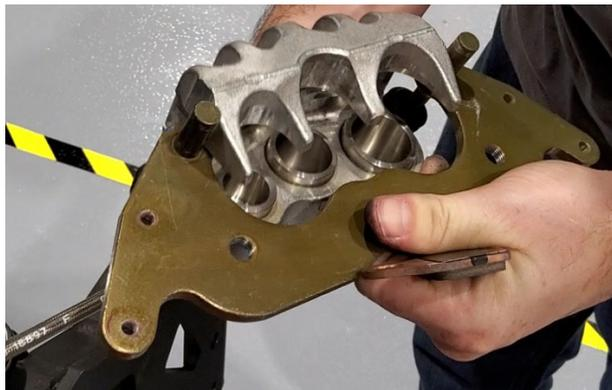
Remove the stock hanger bracket from the caliper.
