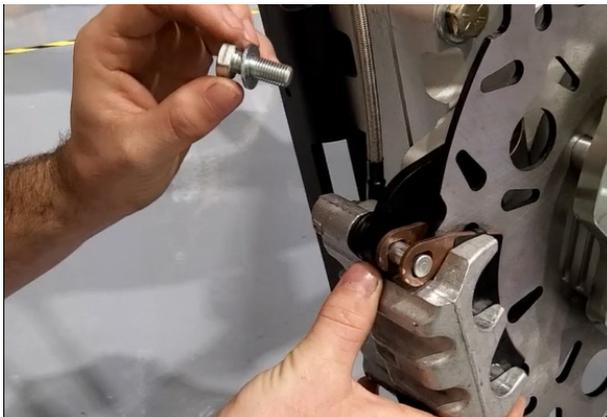
Reconnect the line and Install the caliper onto the portal box. Use the **10x25 bolts** with **10 mm washer** to secure the caliper to the bracket [30 ft lbs]. (These replace the factory 50mm bolts)
