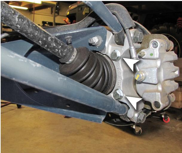
**Remove the brake caliper mounting bolts from the hub assembly (15mm). Set Brake caliper aside.**
