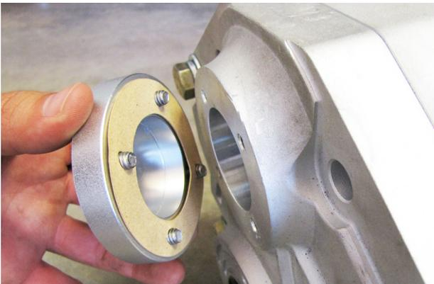
Remove the 1/4-20 x 3/4" screws & cap/gasket from the lid of the portal box.
