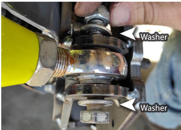
Use a 12mmx 65 bolt to secure a radius bar. Install a 12mm washer on each side and secure it with a 12mm lock nut. (18mm) [90 ft lbs].
