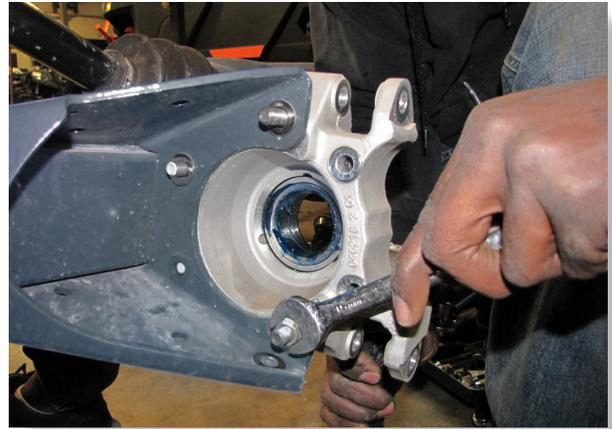
Remove the bolts and nuts that secure rear knuckle to the TRAILING ARM (15mm) Remove the rear knuckle.
