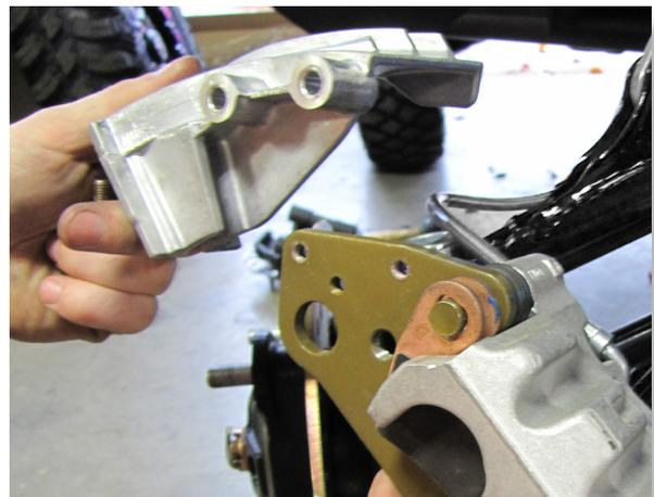
Remove the **brake caliper mounting bolts (15mm)**. Remove the **front mud scraper (8mm)**. **KEEP ALL FACTORY HARDWARE. DO NOT REMOVE BRAKE LINE.** Set caliper aside.
