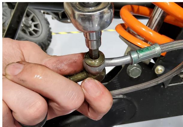
Disconnect the stock brake line from the caliper. Have a container ready to collect brake fluid. Locate the proper BRAKE LINE EXTENSION. Using the supplied button head hex drive banjo bolt, connect the STOCK BRAKE LINE to the BLIND-END BRAKE LINE EXTENSION. Ensure the copper washers are on each side of the banjo fitting.
