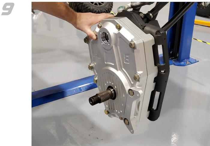
Apply **water-resistant grease** to the **drive splines**. Be sure to apply product all around the outer edge as well.
