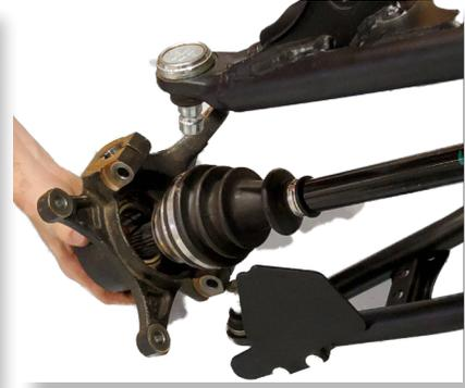
Disconnect the **Lower ball joint** by removing the bolt at the knuckle (15mm).
