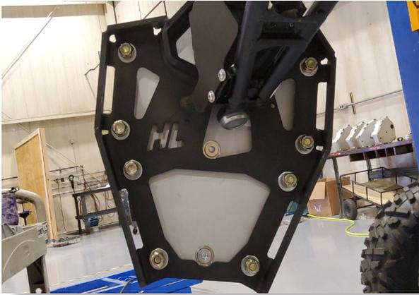
Insert the bolts through the corresponding holes in the backing plate.
