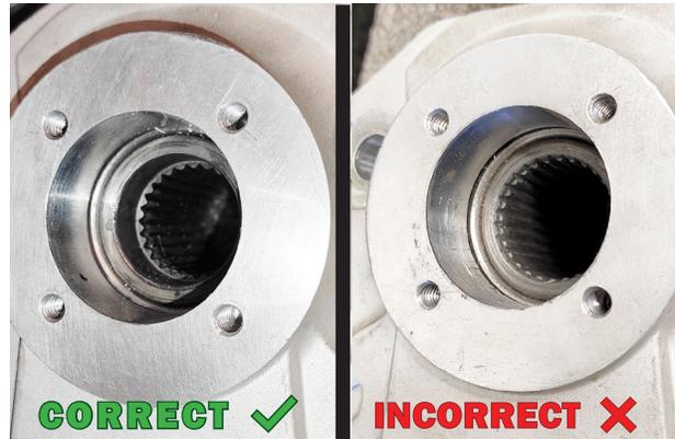
**NOTE:** On the FRONT & REAR portal boxes, the drive gear splines should be recessed to accommodate the shorter front drive shaft splines.
