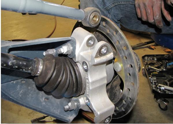
Remove the bolts and nuts that attach the rear knuckle to the UPPER & LOWER RADIUS BARS (15mm).
