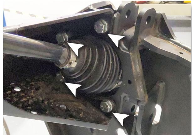
Install the backing plate to the trailing arm using M10 x 35mm bolts and 10mm flat washer on each side. Then fasten bolts with M10-1.25 lock nuts. (15mm) [56 ft lbs].
