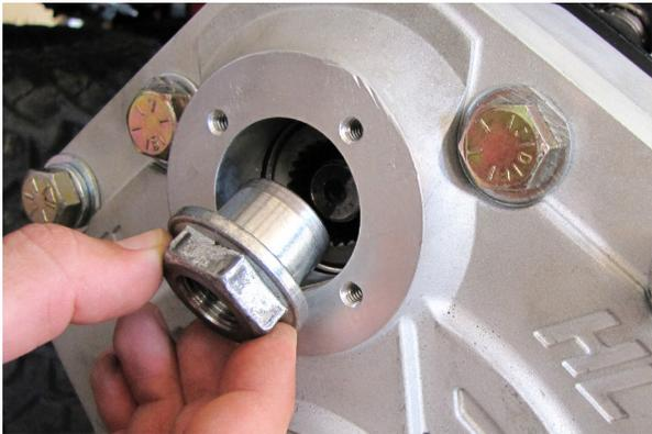
Apply LOCTITE (BLUE) to the supplied M18 axle nut with shoulder PGLC-AXNUT-4 and torque onto the drive shaft axle. (30mm) [20 ft lbs].
