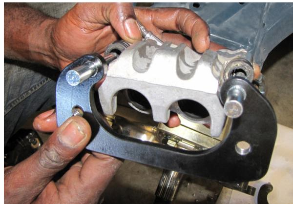
Remove the stock hanger bracket. Install the **85X hanger bracket** into the brake caliper.
