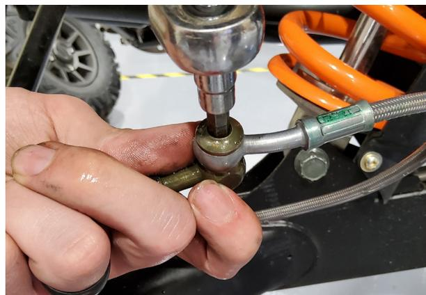
Locate the proper BRAKE LINE EXTENSION. Using the supplied button head hex drive banjo bolt, connect the STOCK BRAKE LINE to the BLIND-END BRAKE LINE EXTENSION. Ensure the copper washers are on each side of the banjo fitting.
