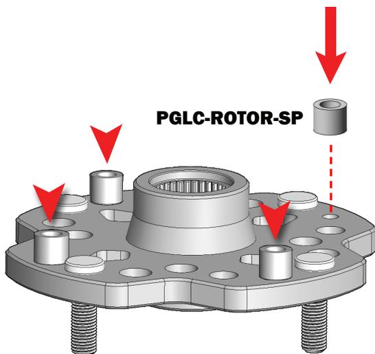
Place the 1/2 spacers over the tapped holes. These spacers go **BETWEEN** the hub and rotor.
