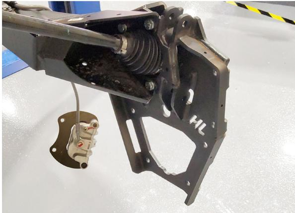
Place the backing plate into position on the trailing arm and guide the drive shaft through.
