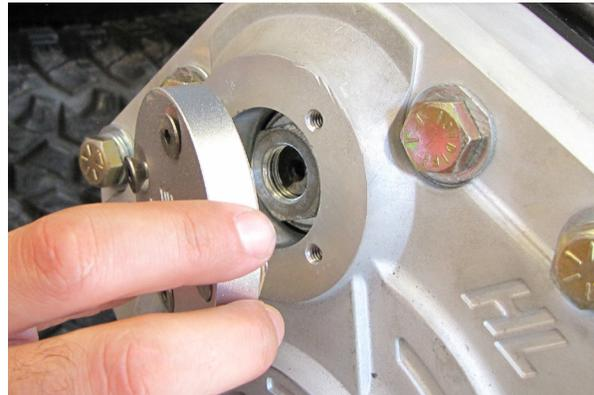
Align the portal box lid cap & gasket. Use the 1/4-20 x 3/4" screws and install the cap to the portal box [8 ft lbs].
