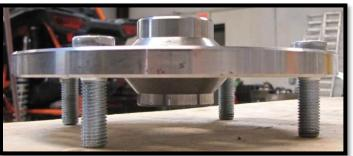
e. Once the studs are pressed in, place (4) 1/2" brake rotor spacers PGLC-ROTOR-SP over the tapped holes.
