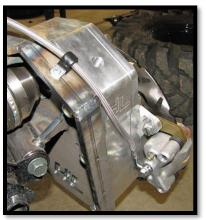
k. Secure brake lines by using the provided **zip ties**. Make sure there is no binding in the lines once they are secured.
