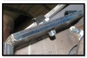
i. Secure the remaining brake line slack by using the **zip ties**. Make sure there's no binding in the lines once they're secured. (Re-using the factory loom clamps is optional, but you may need new hardware/ rivets)
