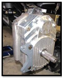
d. Loosely fasten the all four bolts with 1/2" flat washers and 1/2" lock nuts. Recheck all parts that were used and make sure everything fits correctly, and then go ahead and tighten and torque all bolts. (3/4)[105 ft lbs]
