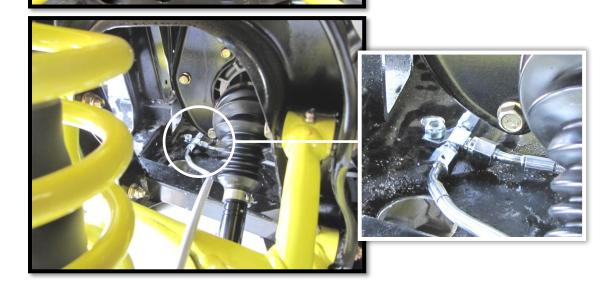
i. If you are installing 6" portals, you must route the brake lines down the inside of rear lower arms to gain enough slack.
