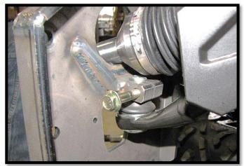
c. Then place the upper ball joint into the upper ball joint mount bracket. Fasten it with the factory hardware. (18mm)[50 ft lbs]
