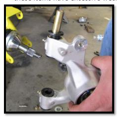
c. Insert the bushings & pivot tubes into the collars of the rear right backing plate (105M-R).
