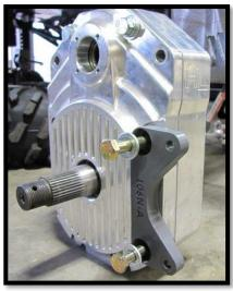
d. Slide a 1/2" flat washer onto (4) 1/2 x 4-1/2" bolts and insert them into the remaining four holes of the box.
