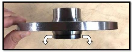
c. With the shorter lip side faced down, find the bolt pattern that corresponds to your make and model. Use the provided studs PGLC-WSTUD-103 (10mm-1.25 stud) (4/137mm bolt pattern)
