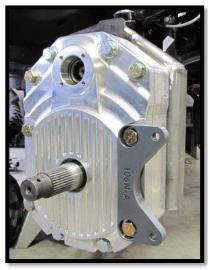
d. Loosely fasten the all six bolts with 1/2" flat washers and 1/2" lock nuts. Recheck all parts that were used and make sure everything fits correctly, and then go ahead and fasten all bolts. (3/4)[105 ft lbs]
