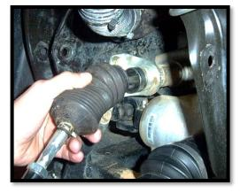
d. Place the steering stop clips (2ea) between the inner tie rod joint and the rack and pinion. It is a tight fit, so you may have to force it on this is to ensure that the spacer stays in place.
