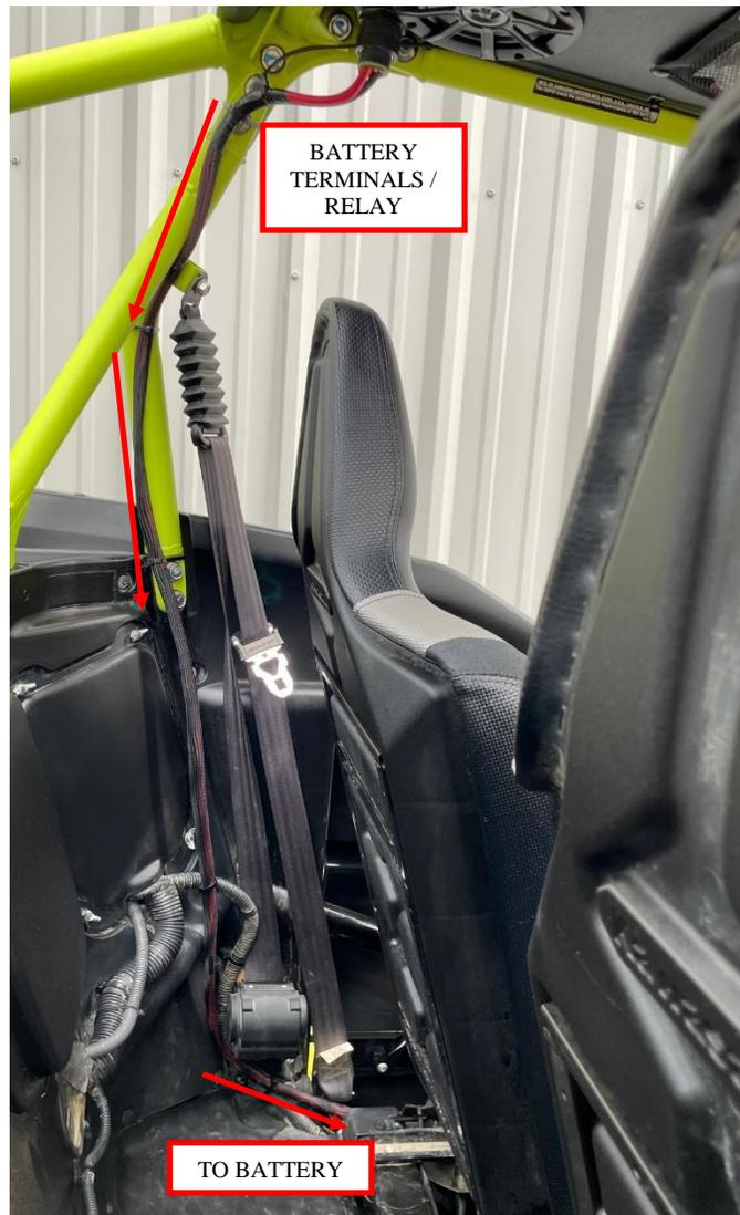
**Figure 11: Route the battery ends and relay to the battery under the driver's seat.**
