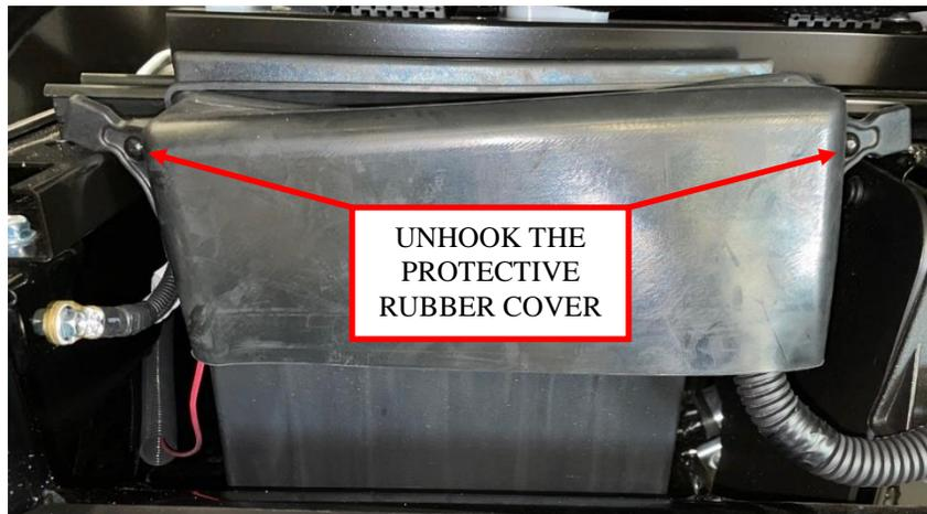
**Figure 12: Remove the protective battery cover.**
