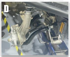
REPEAT STEPS ON OTHER SIDE THEN REINSTALL WHEELS AND LOWER THE JACK. YOU WILL NEED TO ADJUST THE TOE.
