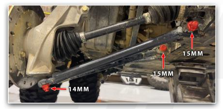
THESE ARE THE THREE BOLTS AND NUTS PER SIDE TO BE REMOVED FOR THIS INSTALLATION.
