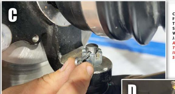
CHECK THAT EVERYTHING FITS CORRECTLY AND TIGHTEN ALL NUTS TO SPEC. REINSTALL THE WHEELS AND LOWER THE JACK. YOU WILL NEED TO ADJUST THE TOE. REFER TO THE BACK OF THE INSTRUCTIONS FOR THE STEPS.
