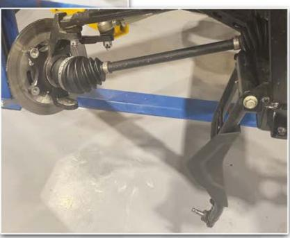
NOW REMOVE THE LOWER CONTROL ARM BY REMOVING THE FACTORY 14MM BOLT AND NUT.
