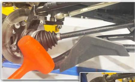
YOU CAN USE A RUBBER MALLET TO STRIKE THE LOWER ARM LOOSE FROM THE KNUCKLE.
