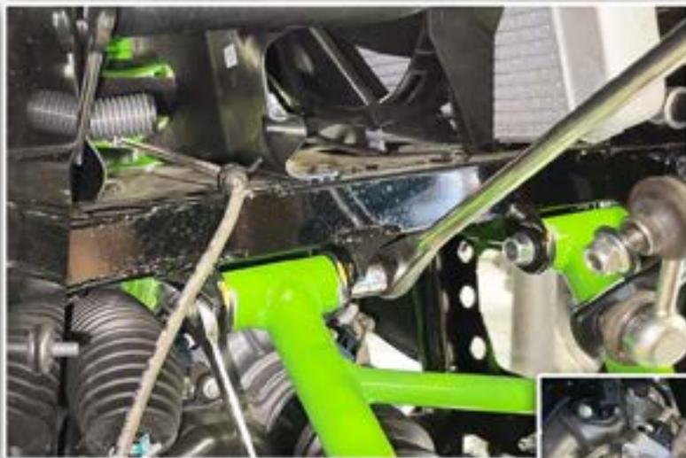
**NOW REMOVE THE BOLTS AND NUTS HOLDING THE UPPER ARM TO THE FRAME. (17MM)**
