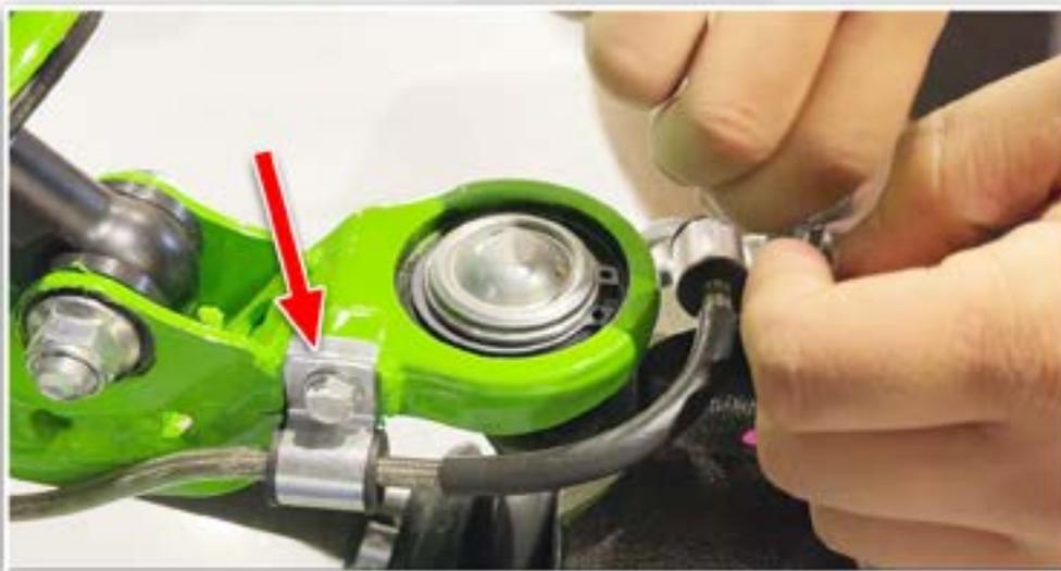
REMOVE THE 4 (10MM) BOLTS THAT RUN UP THE A-ARM HOLDING THE P-CLAMPS ON SO YOU CAN MOVE THE BRAKE LINE OUT OF THE WAY.
