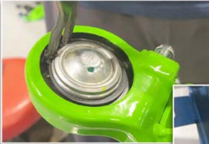
FIRST REMOVE THE RETAINING CLIP. YOU WILL NEED A PRESS AND A SOCKET THAT IS THE SAME DIMENSIONS AS THE BALL JOINT TO PRESS THE BALL JOINT OUT.
