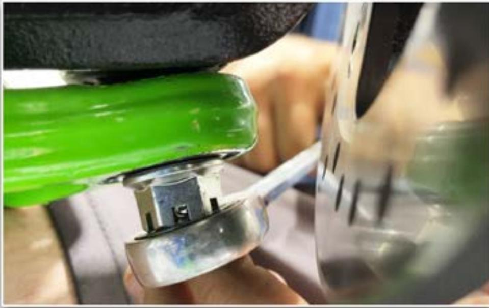
**REMOVE THE LOWER A-ARM AT THE KNUCKLE.**
