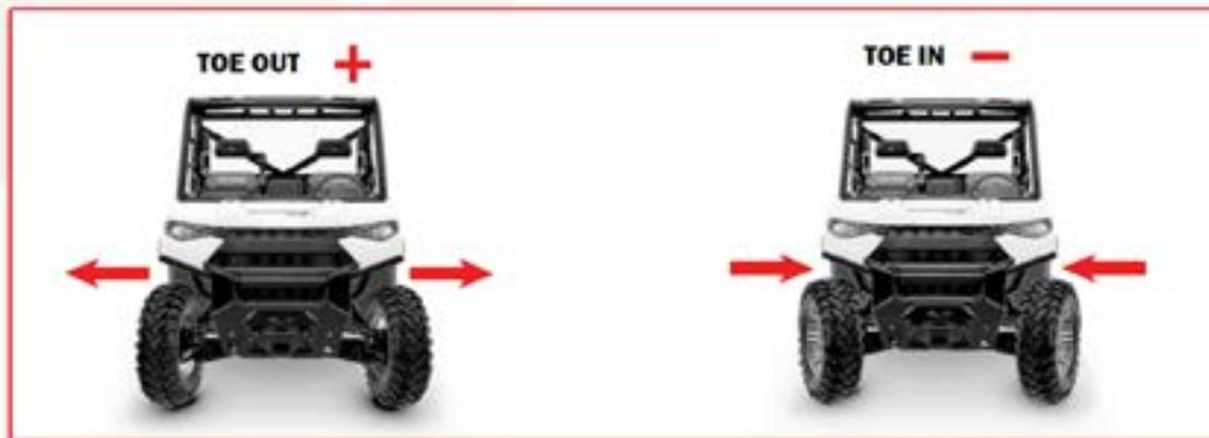
IF THE FRONT OF THE WHEELS ARE POINTING OUT, ADJUST THE TIE RODS **OUT** OR **INCREASE THE LENGTH OF THE TIE ROD**. MEASUREMENT AT THE FRONT OF THE TIRES WILL BE GREATER THAN THE REAR, IF THE TOE IS OUT.
