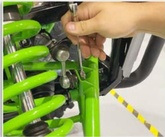
**REMOVE THE FACTORY SWAY BAR NUT. (14MM)**
