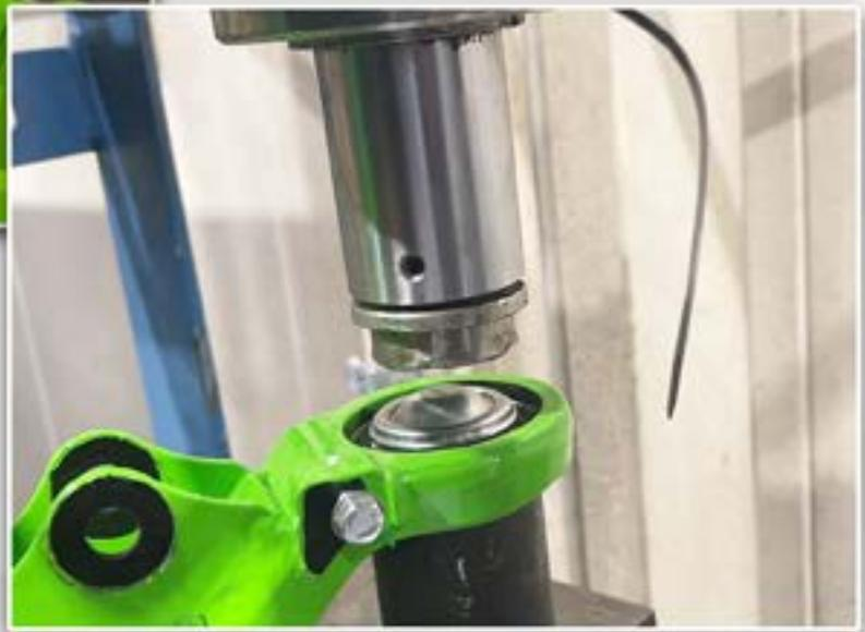
NOW SET THE BALL JOINT INTO THE NEW ARM AND PRESS IT INTO PLACE USING THE SAME SOCKET AS BEFORE.
