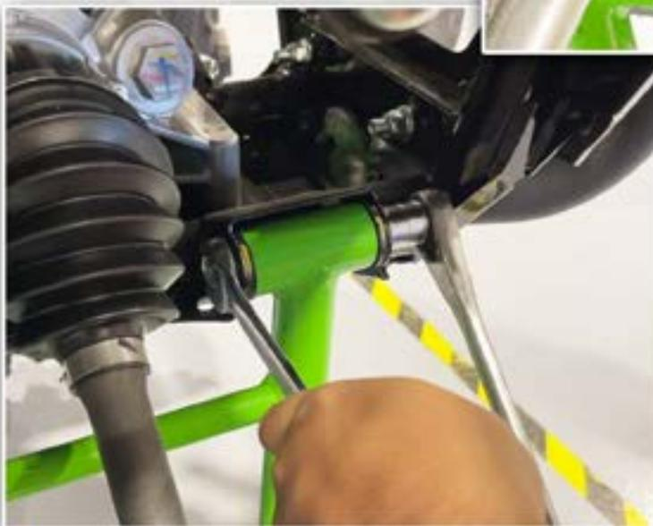
THEN, REMOVE THE (17MM) NUTS AND BOLTS HOLDING THE LOWER A-ARM TO THE FRAME.
