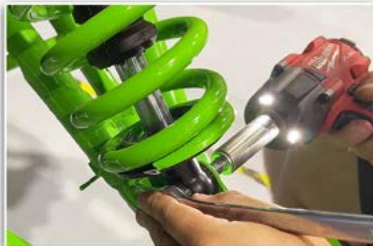
**NEXT, REMOVE THE BOLT AND NUT FROM THE SHOCK TAB. (17MM)**
