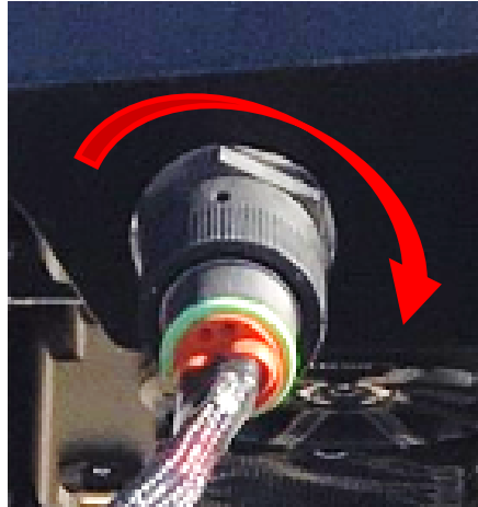
Figure 15: Align connector terminals and rotate 1/4 turn.
