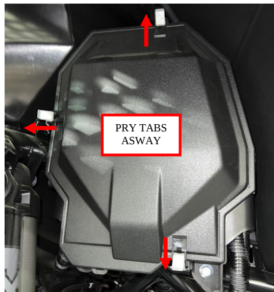
Figure 7: Remove the battery cover.
