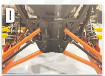
CHECK TO SEE THAT EVERYTHING FITS THEN TIGHTEN BOLTS TO FACTORY SPECS. REINSTALL WHEELS AND LOWER THE JACK.
