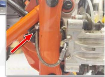
ONCE ALL THE BOLTS ARE REMOVED REMOVE THE FACTORY PLATE AND THEN INSTALL THE TOW HOOK USING THE FOUR FACTORY BOLTS AND NUTS.
