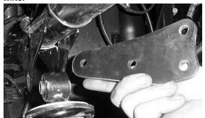
5) Insert it through the stock shock mount, but place a (1.241") spacer between the shock tabs.
