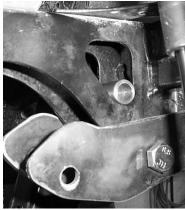
7) Rotate the brackets back up and insert a 12x80mm bolt through the brackets and spacer.
