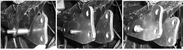
7) Next insert a **(1.537")** spacer to the back, between the lift brackets. Insert a 10x65mm bolt through the brackets and spacer. Fasten loosely with a 10mm lock nut.
