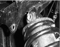
4) Connect two of the front lift brackets to the UTV. Insert a 10x65mm bolt through the lift bracket in the center hole.
