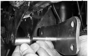
6) Place another lift bracket on the opposite side and loosely fasten it using a 10mm lock nut.
