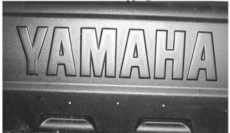
4. Using the self tapping screws provided, attach the logo plate to the tail gate.
