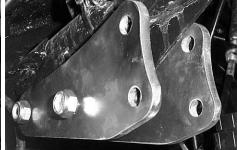
To the front of the lift brackets insert a (1.537") spacer between the lift brackets. Insert a 10x65mm bolt through the brackets and spacer. Fasten loosely using a 10mm lock nut.
