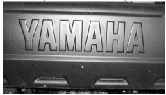
3. Take the logo plate and center it on the mark and mark the holes for the self tapping screws.
