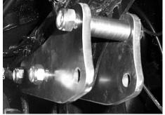
9) Connect the shock to the brackets. Insert a 10x65mm bolt through the bracket, place 2ea 10mm washer on either side of the shock eyelet, insert bolt through and fasten tight using a 10mm lock nut.
