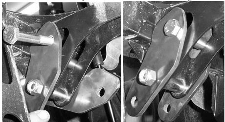
8) Attach the top of the shock to the lift brackets by placing a **(0.2645")** spacer on either side of it between the sock and brackets. Use a 12x80mm hex bolt and 12mm lock nut.
