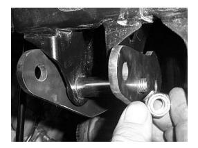
6) Let the brackets rotate down so that you can insert (2.214") spacer above the stock shock mounting location between the frame.
