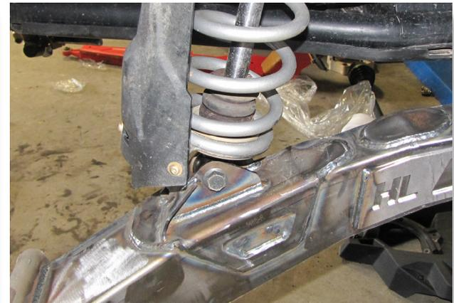
Secure the shock to the trailing arm using factory hardware.
