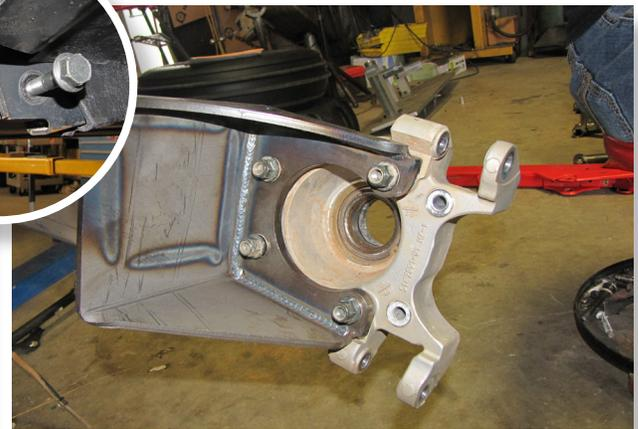
Secure the knuckle to the trailing arm by using the factory (4) nuts & (4) washers (17mm) USE TOE SHIMS HERE TO MAKE CAMBER CORRECTIONS.
