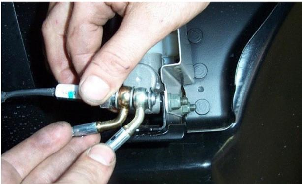
Disconnect the banjo bolt and brake lines from the master cylinder.
