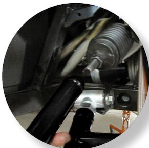
Install the boot over the (HL-TRE-002) inner tie rod, then thread on the tie rod (151H) to the inner tie rod end.
