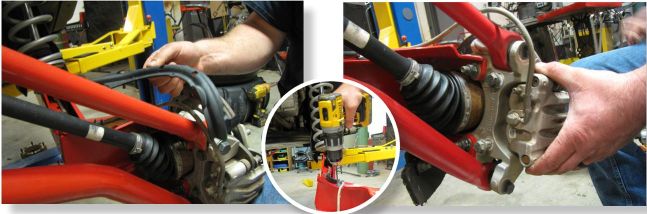
Remove the brake line guard by removing the bolts securing it.
