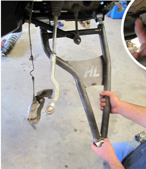
Connect the lower arm at the frame. **USE FACTORY HARDWARE.**
