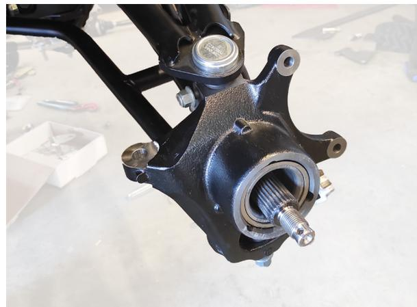
Remove the **cotter pin**, **axle nut**, and **washers** from the hub assembly, then remove the hub. (27mm) **KEEP FACTORY HARDWARE.**
