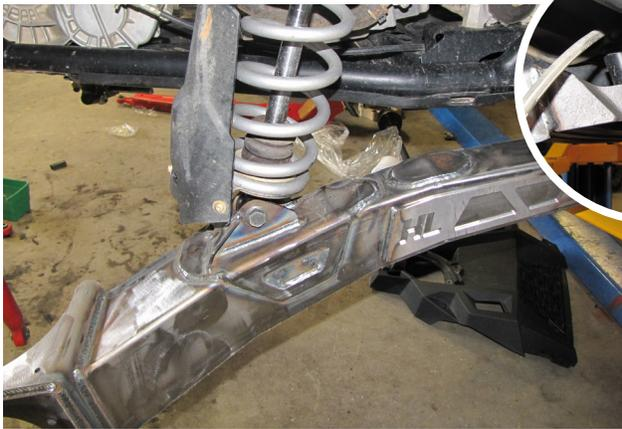
Install the new trailing arm to the frame, use factory hardware to secure.
