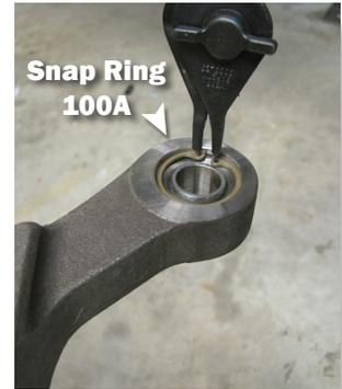
Once the bearing (31J) is in place, use a socket of the same diameter as the outer race to press it in all the way. Apply grease to outer race to ease install.
