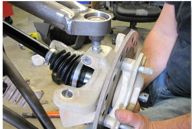
Slide the axle through the hub assembly. Connect the lower arm at the knuckle, then the upper arm. Secure with factory hardware.
