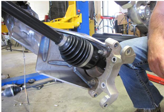
Install the new axle into the rear differential, then slide it into the knuckle.
