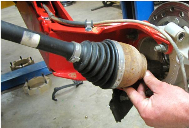
Completely remove the axle by removing it from the knuckle and the differential.
