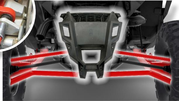
If you cannot access the radius bar mounting bolts due to the plastic bumper, remove it. Remove the nuts and bolts securing the UPPER & LOWER radius bars at the frame and hub.
