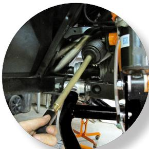
Remove the clamp from the boot, then remove the stock tie rod.
