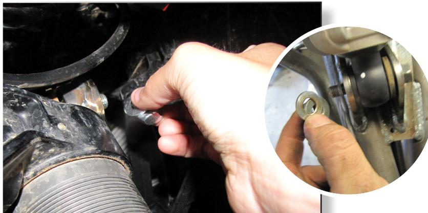
Once the arms are mounted, install the shock. Secure it with a **M10x75mm bolt** through the upper shock lift bracket, then install a **10mm washer** and fasten with a **10mm lock nut**.
