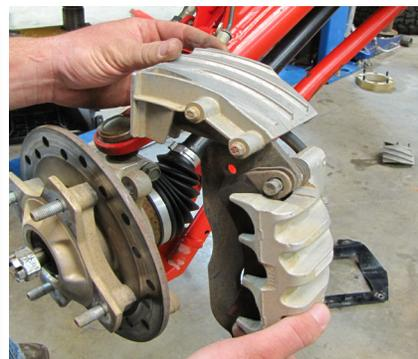
Remove the **brake lines** from arms and frame by drilling off the rivets. Remove the (2) **brake caliper mounting bolts (15mm)** **DO NOT** disconnect lines from caliper. Set brake caliper aside.
