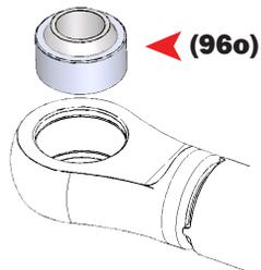
Once the bearing (96o) is in place, use a socket of the same diameter as the outer race to press it in all the way. Apply grease to outer race to ease install.
