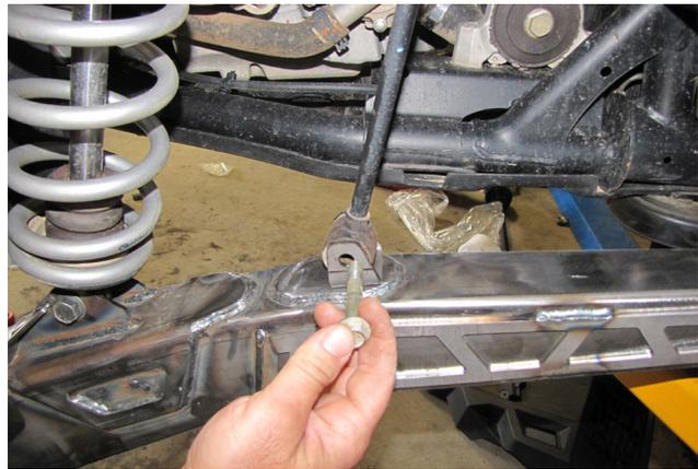
Secure the stability bar in place, use factory hardware.
