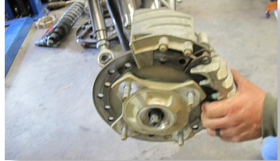
Re-secure fitting to caliper if you have not done so already. Connect the caliper to the hub assembly. (15mm)
