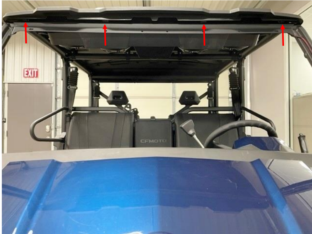
Figure 2: Remove the front bolts securing the roof to the visor.
