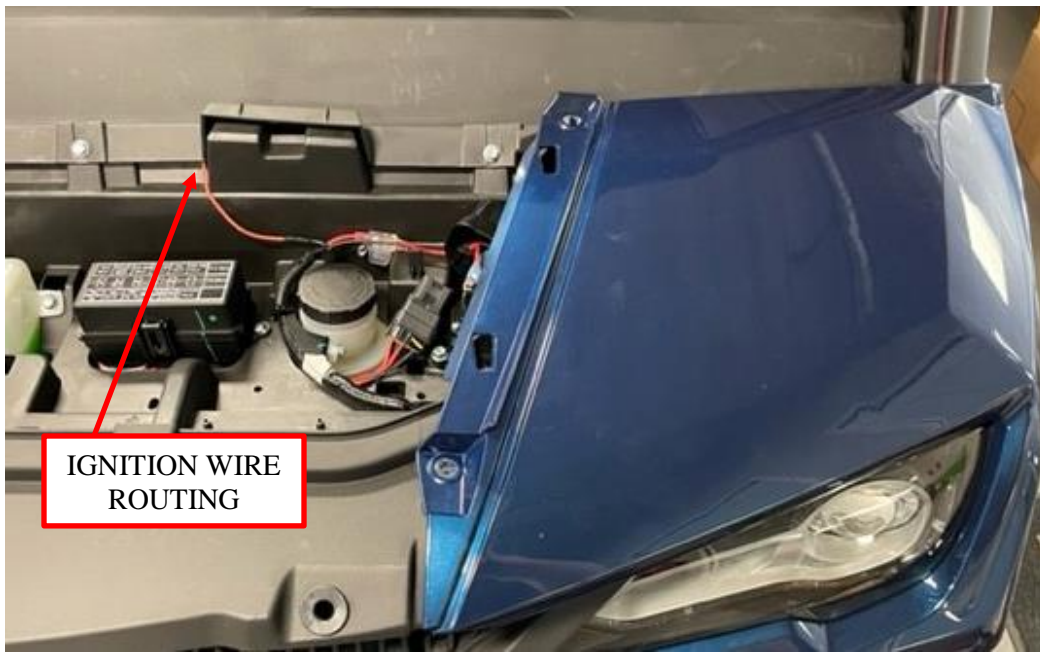
Figure 14: Accessory wire routing for ignition power source under the dash.
