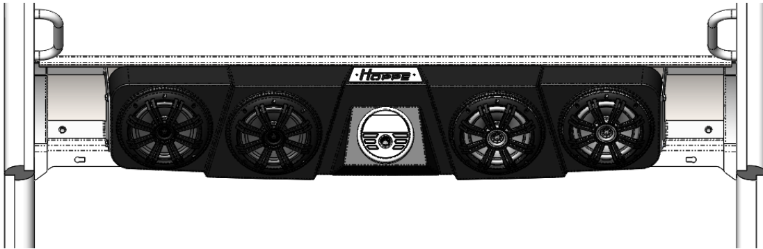
Figure 7: Loosely install the sound system on the mounting brackets.
