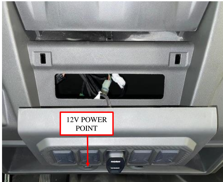
Figure 16: Connect the chassis harness to 12V power point connectors.
