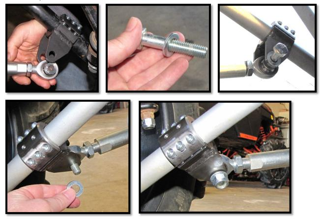
28. <u>Next, you must complete a CLEARANCE CHECK</u>. Follow the steps and check for clearance before riding. If you check before riding you can adjust before you damage the bars, clamps, or other parts.
