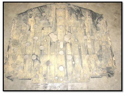
15. Reattach the skid plate over the control arm link plate. Secure the skid plate using the factory hardware.
