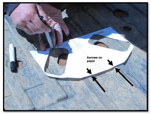
14. Cut the marked sections in the skid plate using an oscillating/cutting tool.
