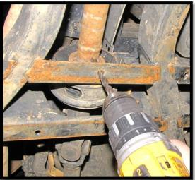
5. Slide a **5/16**" flat washer onto a **5/16**" x **1**" bolt. Then connect the frame plate **93A** to the frame and loosely secure it with the **5/16**" washer and **5/16**" lock nut.
