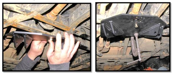
6. This plate is used on multiple kits, so use the bolt holes that are designed for this SXS. See illustration of which holes are used.
