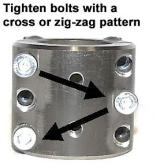
23. Loosely connect the **clamp collars 96R & 96T** onto the lower control arm. Connect it at the lowest point possible on the arm using the **¼-20 x ¾**" **socket head bolts**. <u>Keep in mind you will need to adjust it later, so fasten snug, not all the way tight</u>.
