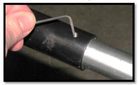
43. Located on each clamp collar are two ¼-20 x 3/8" set screws. Make sure that the set screws are tighten so that the collars cannot move during use.
