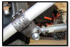
42. Located on each (hollow) bar is a single **%-28 x 3/16**" set screw. Make sure that the set screw is tight so that the bars will not rotate during use. Do not over torque.
