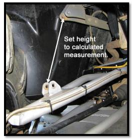
36. Use a jack stand or a friend to hold it in place while you situate the link bar to be close but not touching the frame. You can adjust the bars, slide the clamp up and down on the control arms, and rotate the collar to achieve proper clearance.
