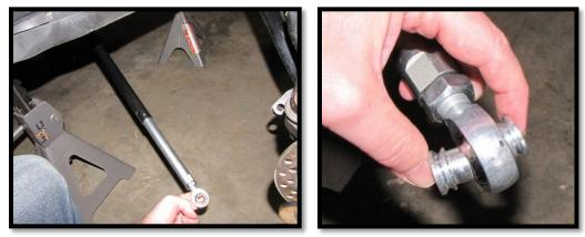
27. Connect the heim joint to the collars on the control arms. Place alignment cones on either side of the heim joint. Connect to the collar using the ½" x 2-3/4" bolt, 12mm washer 2ea, and ½" lock nut. Torque the nut to 110lb-ft. Repeat to the other side.
