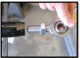
19. Now insert the two **alignment cones 96Q** into to the eyelet of the heim joint and connect it to the plate.
