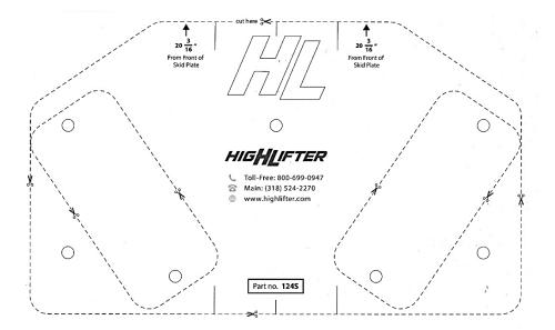
12. With the skid plate lying flat with the <u>frame side down</u>, use a tape measure and measure 20-3/16" down from the front edge of the skid plate. See the illustration in image of where to start your measurement.
