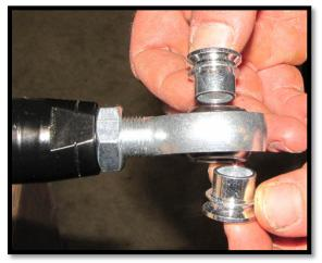
20. Connect the heim joints to the plate using the ½" x 2-3/4" bolt, 12mm washer 2ea, and ½" lock nut. Torque the nut to 110lb-ft.
