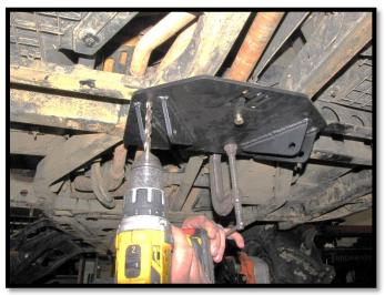
9. Slide a **5/16**" **flat washer** onto (4) **5/16**" **x 1**" **bolts** to connect the plate to the frame. Loosely secure them with **5/16**" **flat washers** and **5/16**" **lock nuts**. Torque bolts to 25lb-ft.
