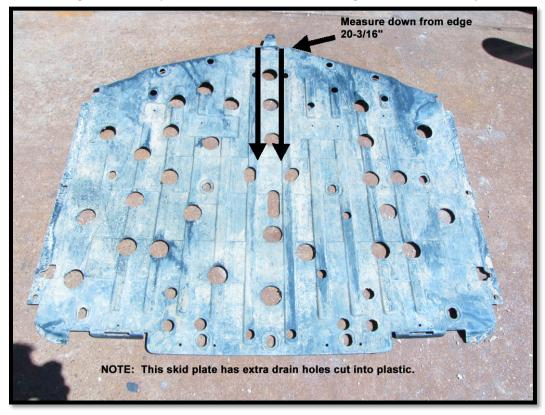
13. Located on the top and bottom edges of the template are three lines. Two long and one short. Use these lines to center the template on the ribs of the skid plate. The two longer lines go to the inside edges of the two center ribs and the one single line is the center between the two ribs. Once you have aligned the upper and lower lines on the template mark the hole to be cut in the skid plate.
