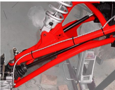
When you have completed the brake line installation, reconnect the lines to the calipers. Use the factory hardware to reconnect all lines.
