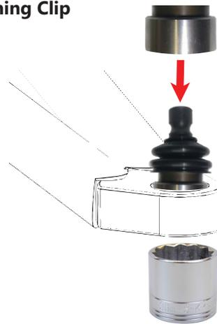
Back the ball joint with a large 36mm socket or something sturdy of similar diameter, then using a press or vice, press the ball joint out of the arm.
