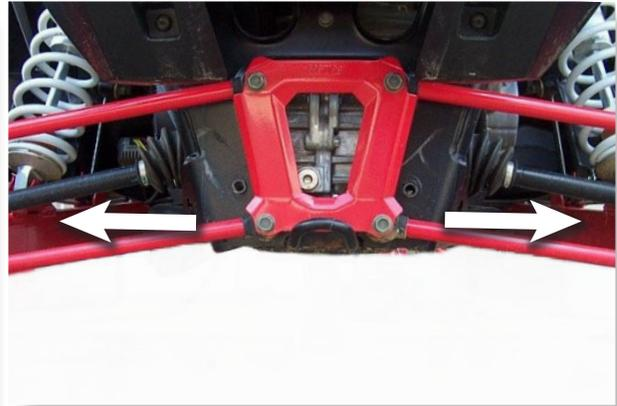
Remove the factory axles from the differential.
