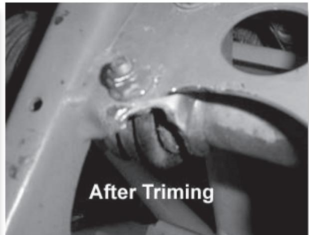
Trim the frame so that the pinion has proper clearance.
