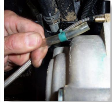
Reconnect wires and vent lines to the differential.
