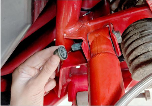
Once bushings and ball joints are installed, connect the new upper arm to the frame using the factory hardware. **DO NOT FORGET WASHERS.**
