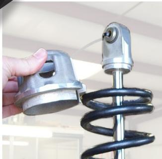
Compress the spring and remove the retaining collar from the shock.
