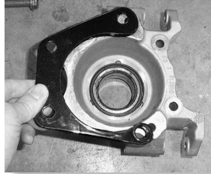
Remove the hub assembly from the trailing arm. **KEEP ALL FACTORY HARDWARE.**
