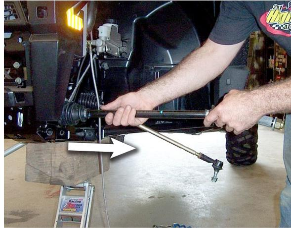
Now pull the axle out of the differential. You may need to tug hard on the axle to pop it out of the differential.
