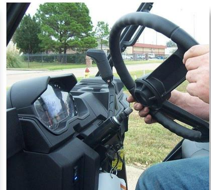
Once the nut is broke, back it off just enough leaving a few threads. Use a hammer to tap on the nut while pulling up on the steering wheel until it breaks loose. But **DO NOT** hammer too hard, it could damage the nut or threads. Now remove the nut and steering wheel.
