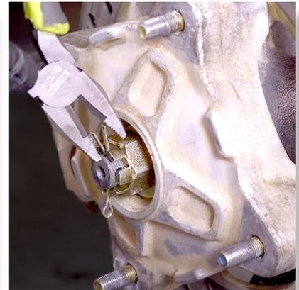
Remove the **cotter pin** and **castle nut** that secures the axle to the **knuckle assembly**.
