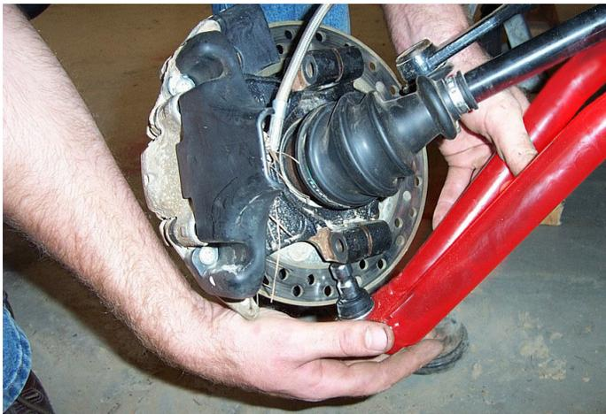
Attach the control arms to the knuckle assembly where the pinch bolts are, by using the factory hardware. **DO NOT FORGET WASHERS.**
