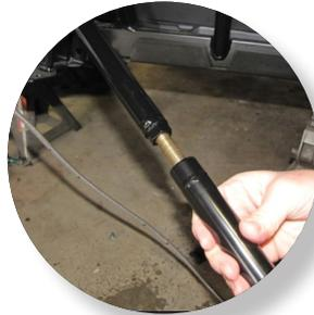
Thread on the tie rod extension and tighten it.
