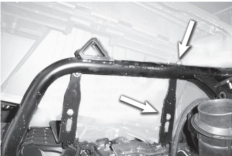
There is a support bracket that needs to be unbolted to allow for the lift bracket to slide into place. Unbolt the bracket, slide the lift bracket into place, then reattach the factory bracket. Remove and set bracket aside, then slide the lift bracket into place and attach it.
