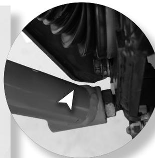
It may be necessary to trim the trailing arm to gain the desired clearance for the lower radius bar.
