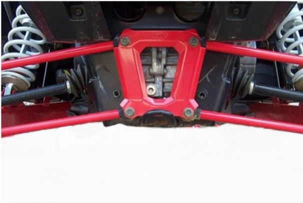
Disconnect the stock upper and lower radius bars from the frame.
