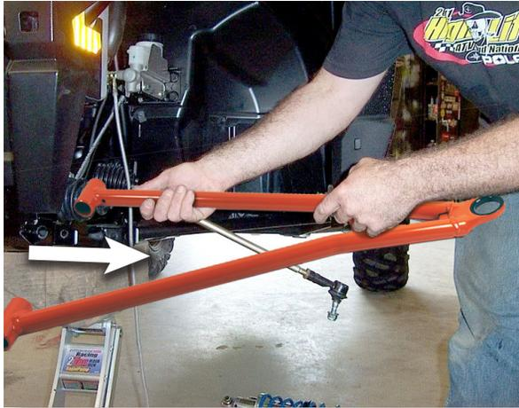
Disconnect the **upper and lower control arms** from the frame. Do this on both sides.
