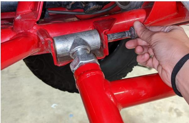
Once the ball joints are installed, connect the new lower arm to the frame using the factory hardware. **DO NOT FORGET WASHERS.**
