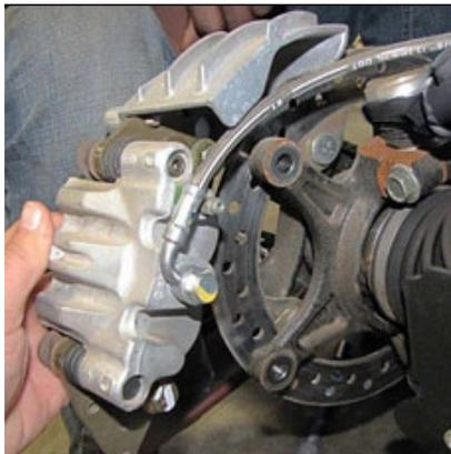
Disconnect the **calipers** from the knuckles and the brake lines from the A-arms. Place the calipers aside.
