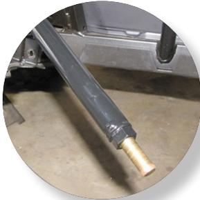
Slide the tie rod sleeve over the factory tie rod.
