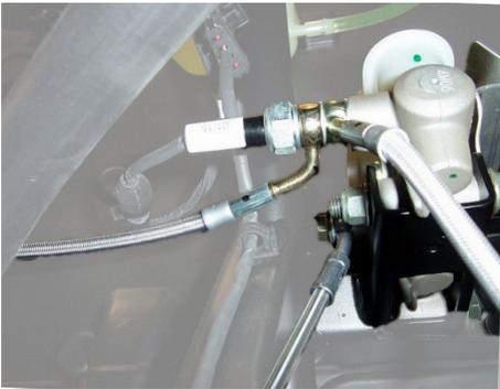
Before you proceed with the installation of the lift kit and new control arms, you will need to **disconnect the brake lines from the master cylinder**. You are going to take the factory brake line on the **PASSENGER** side of the RZR and install it on the **DRIVER** side. The new 45X brake line will be attached on the right side of the RZR.
