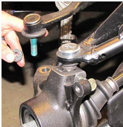
Disconnect the **tie rod** from the **knuckle assembly**.
