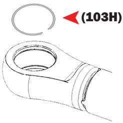
Insert a c-clip (103H) into one side, then place a spherical bearing (96o) into the other side.
