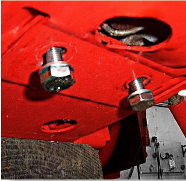
Secure the rear shim to the differential.
