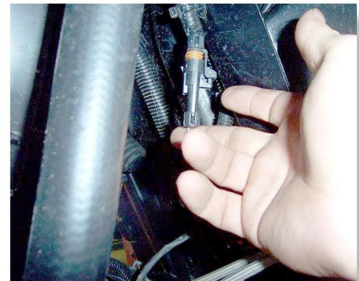
Disconnect the **wires and vent line** from the **front differential**; then remove the **4 bolts** that secure the differential to the frame.
