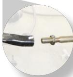
Disconnect outer tie rod end & remove jam nut.
