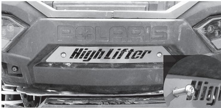
Using the two 5/16 x 1" button head bolts, 5/16" washers and 5/16" lock nuts connect the logo plate to the rear plastic and reattach the plastic.
