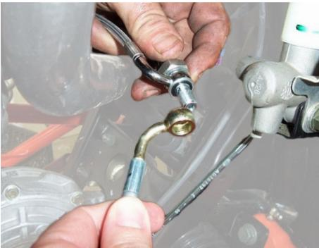
Disconnect and remove the **PASSENGER** side brake line from the master cylinder and replace it with the new line provided. Now install the **PASSENGER** side factory brake line on the **DRIVER** side. When you have installed the front arms you will need to route brake lines to the front of the new a-arms. This will ensure that you have no binding or pinching of the brake lines.
