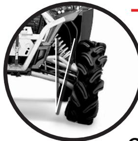
If you have a **positive** camber you will need to adjust the collar **OUTWARD** or **lengthen** the collar. Up to 3° out.
