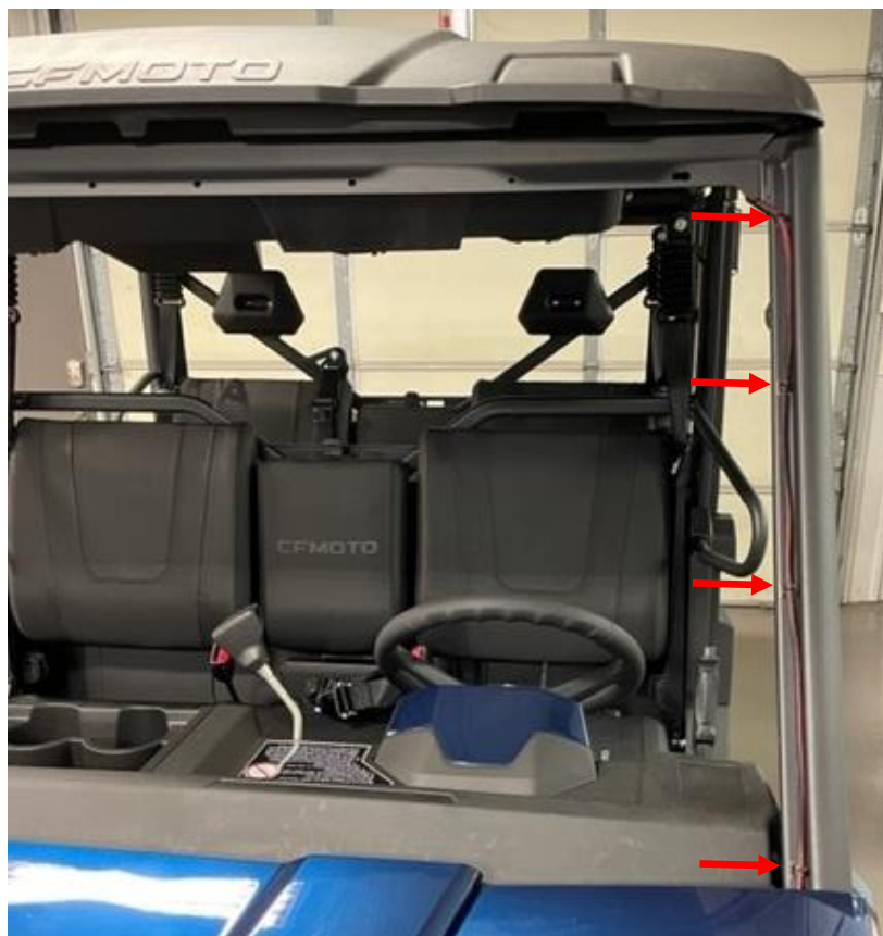
Figure 20: Secure the chassis harness to the frame tube.
