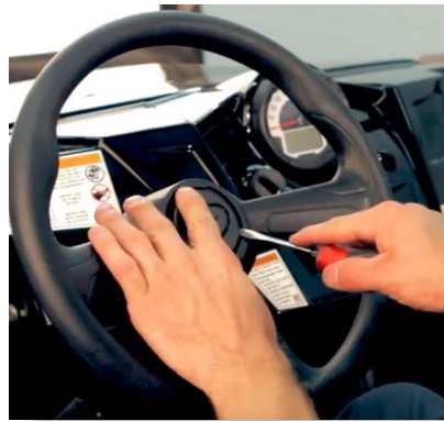
(B) If the steering wheel is not centered, you will need to remove the center cap with a flat head screwdriver to gain access to the steering wheel nut.
