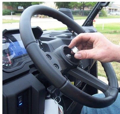
(B) If the steering wheel is not centered, you will need to remove the center cap with a flat head screwdriver to gain access to the steering wheel nut.
