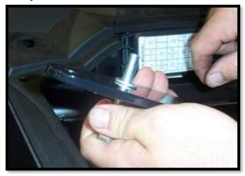
8. Insert the bolt through the shock mount tab. Place a (O) spacer on the bolt between the shock mount tabs. Push the bolt all the way though the shock mount tabs.
