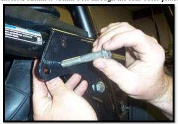
12. Place a (53B) spacer onto the bolt and then connect it to the rear inner plate.
