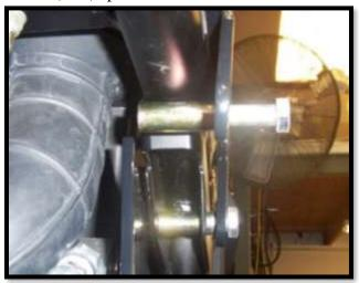
13. Loosely fasten inner lift bracket to the bolt with a 12mm lock nut.
