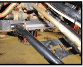
8. Next connect the left and right rear bracket to the control arm tabs. Place a 10mm flat washer on the 10mm x 110mm bolt. Insert the bolt through the brackets and control arm collar. Loosely secure the bolt and brackets with a 10mm washer and 10mm lock nut.
