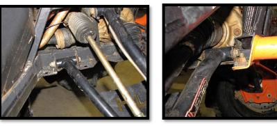
4. If you have a bumper, remove the two bolts that connect the lower portion of the bumper to the frame. These are located near the lower control arms.
