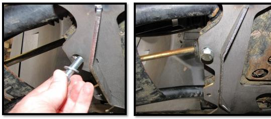
12. On the top side of the frame rail, loosely connect the plate with a 10mm washer and 10mm lock nut. Repeat steps unlit all bolts are in place.
