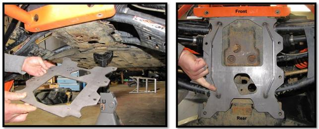
11. Using the 10mm x 35mm bolts, 10mm washers, and 10mm lock nuts, loosely secure the plate to the frame. Place a 10mmm washer onto the 10mm x35mm bolt and insert it into the plate and frame.
